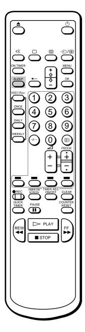
You can automatically switches the video TV into standby mode after a selected time period.
