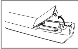
1 Lift the cover at the back of the remote control upward as shown in the figure.
