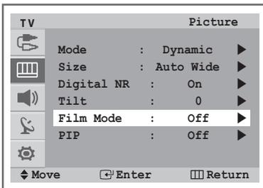
You can automatically sense and process film signals from some sources and adjust the picture for optimum quality.
