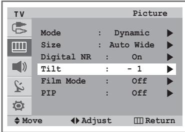
If you find that the picture received is slightly tilted to one side, you can adjust the tilt setting.
