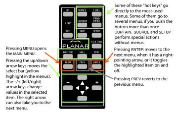
To open menus on the m40L/m46L, aim the remote at the lower right corner (left if portrait) of the screen and press the desired button(s).
