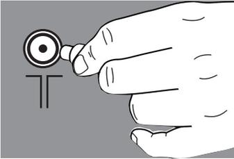
If you use a coaxial cable (round cable) of 75 Ohms as an antenna cable, connect the antenna plug directly to the antenna input located on the TV.
