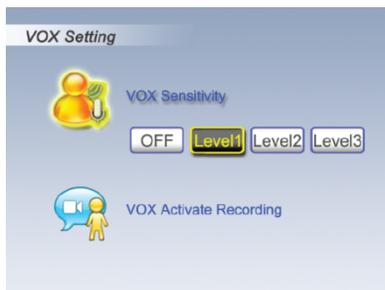
Allows user to set the level of sensitivity for voice activated recording. Level 3 is the highest sensitivity level. This system setting will be set and applies to all cameras while recording.
