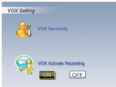
System will auto record for 30 sec once camera is triggered by voice when “VOX Activate Recording” is set to ON.
