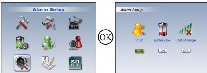
Press **OK** to shift to ON/OFF. Press **◀ ▶** to move between items.
