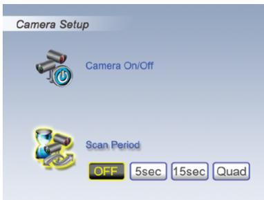
Use ◀ ▶ to change Scan Time interval from OFF / 5 sec / 15 sec / Quad, press Ⓚ to confirm the settings.
