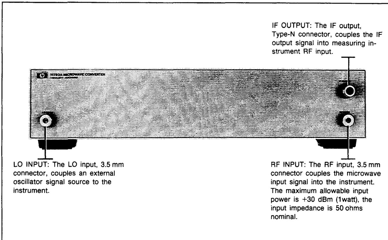
Figure 4. Front-Panel Features
