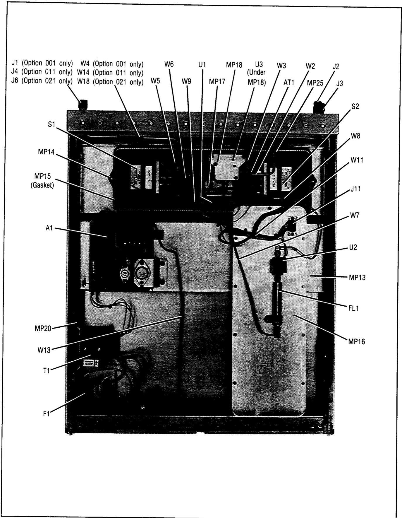
Figure 8. Illustrated Parts Breakdown for Options 001, and 011
