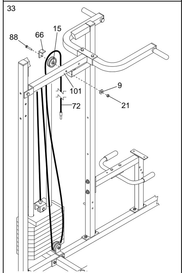
34. See inset drawing A. Attach a 3 1/2" Pulley (15) and a Cable Trap (66) to the upper hole in the Long "U"-Bracket (57) with a 3/8" x 2" Bolt (12) and a 3/8" Nylon Locknut (21). **Be sure that the Cable Trap is inside the Long "U"-Bracket. (Note: This may come pre-assembled.)**
