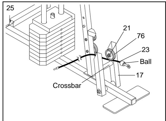
26. Route the Low Cable (23) around the 3 1/2" Pulley (15) attached to the lower hole in the Front Upright (42). **See the inset drawing. Be sure that the Cable Trap (66) is turned to hold the Cable in place and that the Cable is routed around the Pulley as shown.** Tighten the 3/8" Nylon Locknut (21) and the 3/8" x 3 3/4" Bolt (88).
