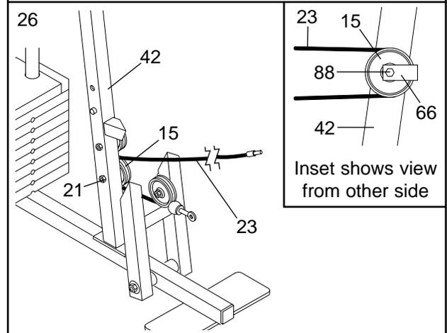
27. Route the Low Cable (23) around the 3 1/2" Pulley (15) attached to the upper hole in the Press Frame (17). **Be sure that the Cable Trap (66) is turned to hold the Cable in place and that the Cable is routed around the Pulley as shown.** Tighten the 3/8" Nylon Locknut (21) and the 3/8" x 3 1/2" Bolt (not shown).
