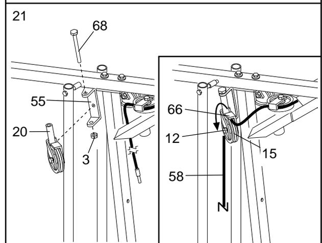
22. See the inset drawing. Attach a 3 1/2" Pulley (15) and a Cable Trap (66) to the upper hole in a Long "U"-Bracket (57) with a 3/8" x 2" Bolt (12) and a 3/8" Nylon Locknut (21). **Be sure that the Cable Trap is inside the Long "U"-Bracket. Note: This may come pre-assembled.**
