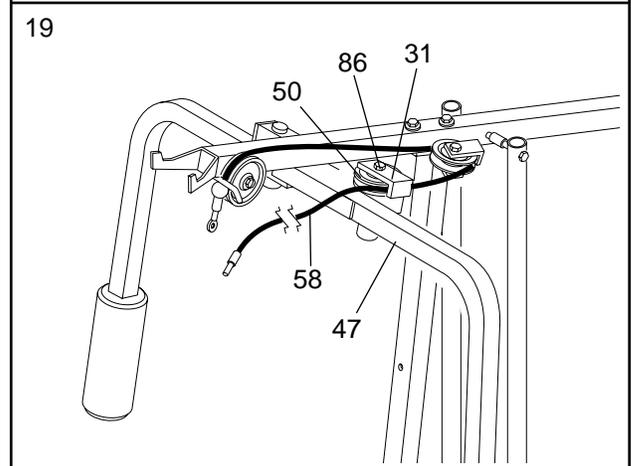
20. Route the High Cable (58) around the “V”-Pulley (50) on the Right Arm (48). **Be sure that the Cable is in the groove of the “V”-Pulley and that the Long Cable Trap (31) is turned to hold the Cable in place.** Tighten the 3/8” x 2 1/2” Bolt (86) and the 3/8” Nylon Locknut (not shown).
