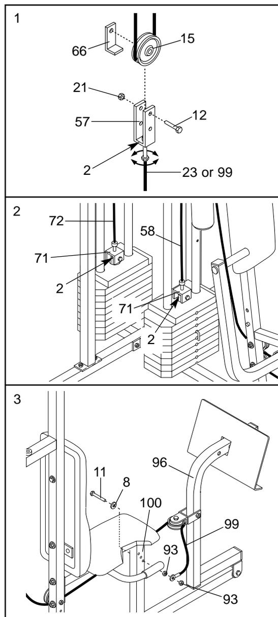
**Do not overtighten the cables. The top weight will be lifted off the weight stack.**
