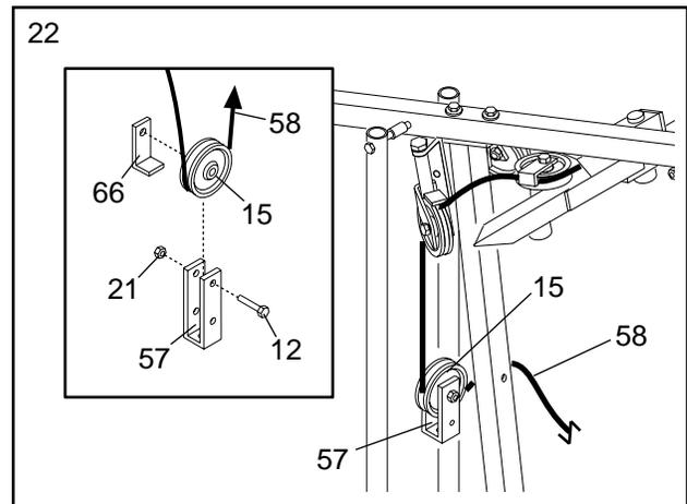
23. Wrap the High Cable (58) around a 3 1/2" Pulley (15). Attach the Pulley to the bracket on the Top Frame (55) with a 3/8" x 2" Bolt (12) and a 3/8" Nylon Locknut (21). **Be sure that the Cable is in the groove of the Pulley and that the Cable and Pulley move smoothly.**
