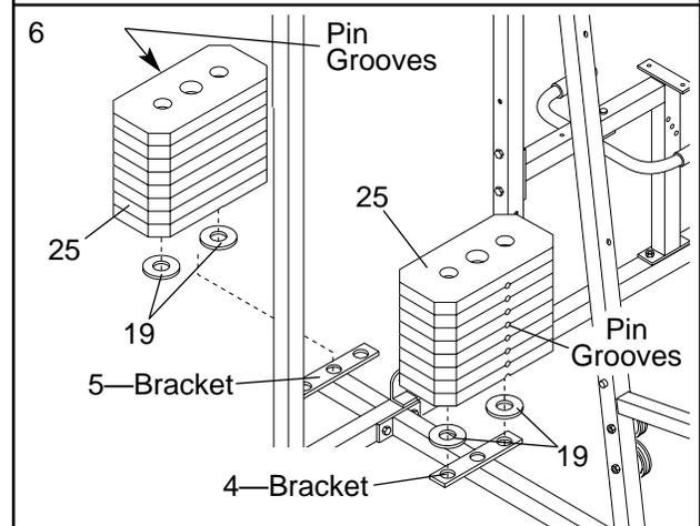
7. Press a Weight Tube Bumper (64) into the end of a Weight Tube (63). Insert the Weight Tube into the front stack of Weights (25). **Be sure that the pin on the Weight Tube is sitting in the pin grooves in the top Weight.**
