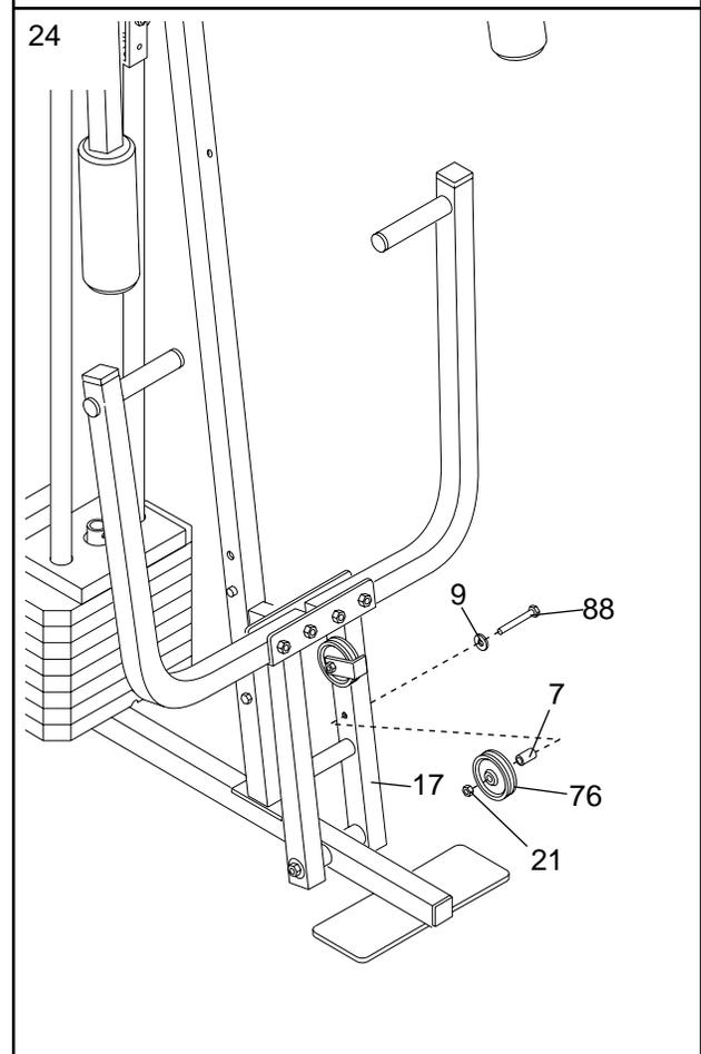
25. **Locate the Low Cable (23).** Route the Low Cable under the 3 1/2" Low Pulley (76) attached to the lower hole in the Press Frame (17). **Be sure that the end of the Cable with the ball is on the indicated side of the Press Frame and that the Cable is between the Pulley and the crossbar on the Press Frame.** Tighten the 3/8" Nylon Locknut (21) and the 3/8" x 3 3/4" Bolt (not shown).
