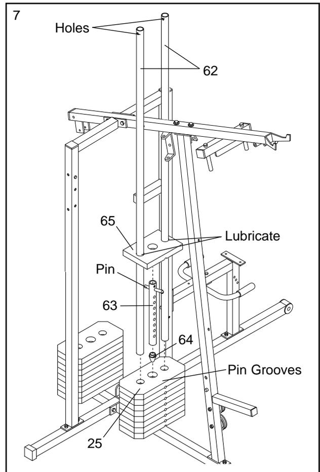
8. Press a Weight Tube Bumper (64) into the end of the other Weight Tube (63). Insert the Weight Tube into the rear stack of Weights (25). **Be sure that the pin on the Weight Tube is sitting in the pin grooves in the top Weight.**
