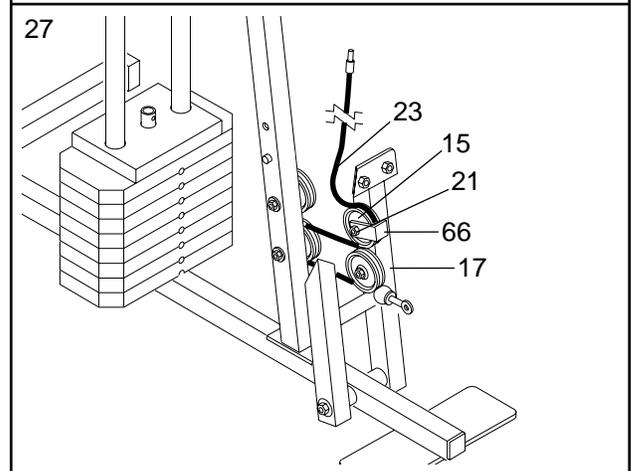
28. Route the Low Cable (23) around the 3 1/2" Pulley (15) attached to the upper hole in the Front Upright (42). **See the inset drawing. Be sure that the Cable Trap (66) is turned to hold the Cable in place and that the Cable is routed around the Pulley as shown.** Tighten the 3/8" Nylon Locknut (21) and the 3/8" x 3 3/4" Bolt (88).
