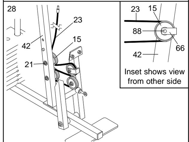
29. Attach the end of the Low Cable (23) to the Long "U"-Bracket (57) with a 1/4" Nylon Locknut (2) and a 1/4" Flat Washer (10). **Do not completely tighten the Nylon Locknut. It should be threaded onto the end of the Cable so only a couple of threads are showing above the Nylon Locknut, as shown in the inset drawing.**
