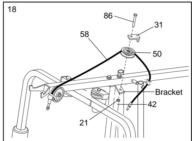
19. Route the High Cable (58) around the “V”-Pulley (50) on the Left Arm (47). **Be sure that the Cable is in the groove of the Pulley and that the Long Cable Trap (31) is positioned to hold the Cable in place.** Tighten the 3/8” x 2 1/2” Bolt (86) and the 3/8” Nylon Locknut (not shown).
