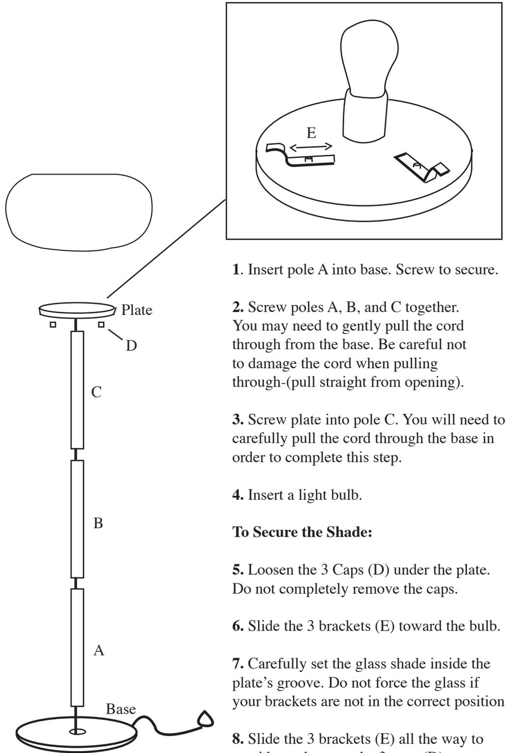
1. Insert pole A into base. Screw to secure.
