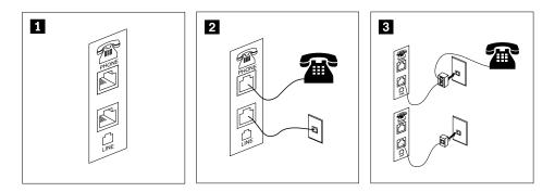
1 This illustration shows the two connectors on the back of the computer that are needed to set up your modem.
