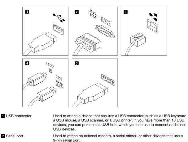
Used to attach an Ethernet cable for a local area network (LAN).
