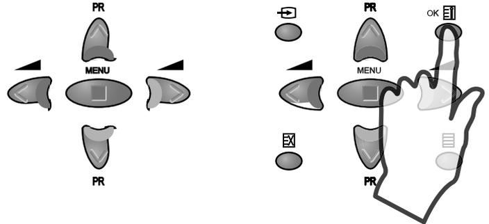
Selection is made by use of the remote control CURSOR UP (A6) / CURSOR DOWN (A21) keys and CURSOR RIGHT (A20) / LEFT (A7) keys.
