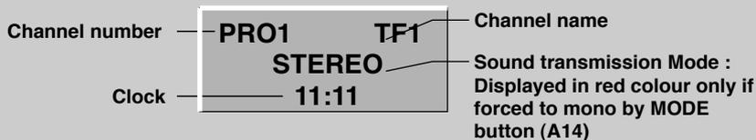
Use the remote control **RECALL** button (A16) to display (for 4 seconds only) program status information. This display appears also after a program selection or after switching on the TV set.
