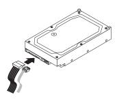
Figure 21. Connecting a SATA hard disk drive
