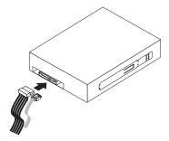
Figure 20. Connecting a SATA optical drive
