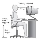
Adjust the monitor so the top of the screen is at, or slightly below, eye level. Place the monitor at a comfortable viewing distance, usually 51 to 61 cm (20 to 24 inch), and position it so you can view it without having to twist your body. Also, position other equipment you use regularly, such as the telephone or a mouse, within easy reach.
