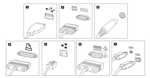
1 USB connector Use this connector to attach a device that requires a USB
