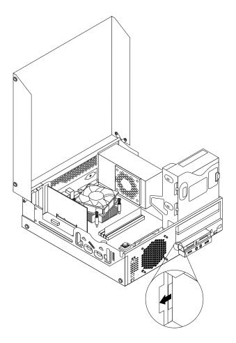
Figure 17. Installing the card reader
