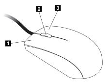
2 Wheel Use the wheel to control the scrolling action of the mouse. The direction in which you
