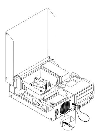
Figure 73. Installing the front WiFi antenna
