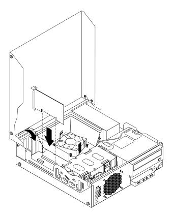
Figure 16. Installing the PCI card
