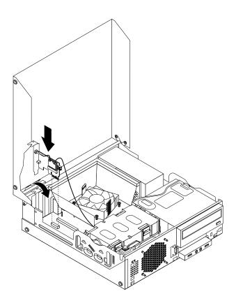
Figure 69. Installing the WiFi adapter card
