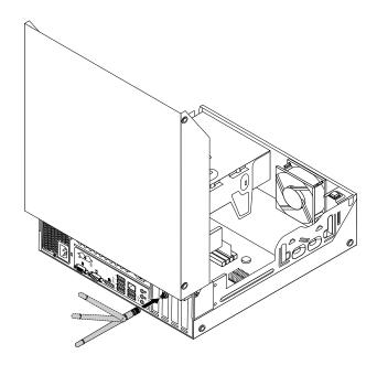
Figure 70. Installing the rear WiFi antenna
