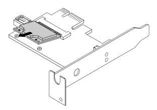
Figure 66. Removing the WiFi card module
