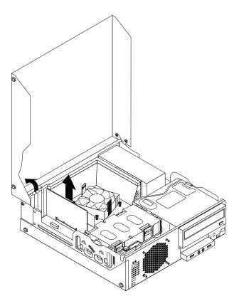
Figure 15. Removing a PCI card
