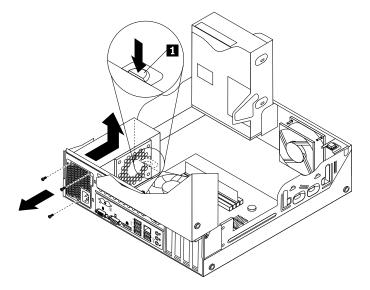
Figure 50. Removing the power supply assembly
