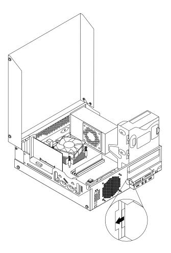
Figure 21. Installing the card reader
