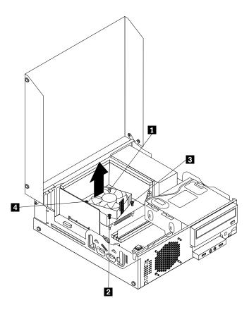
Figure 45. Screws that secure the heat sink and fan assembly
