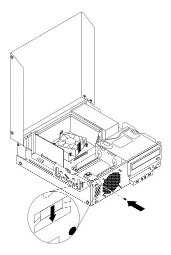
Figure 58. Installing the new cover presence switch
