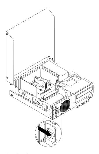
Figure 60. Installing the new internal speaker
