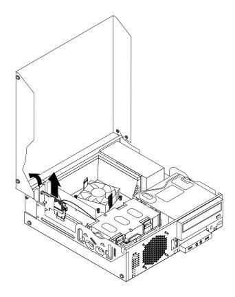
Figure 63. Removing the WiFi adapter card
