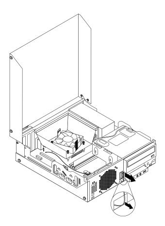
Figure 74. Removing the front WiFi antenna
