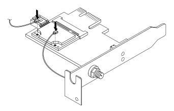
Figure 68. Connecting the WiFi antenna cables
