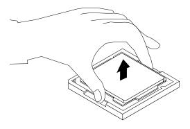
Figure 54. Removing the microprocessor
