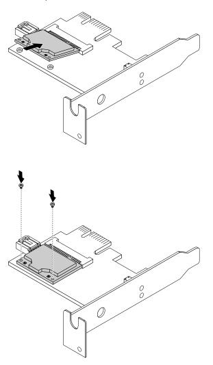
Figure 67. Installing the WiFi card module
