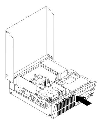
Figure 11. Reinstalling the front bezel
