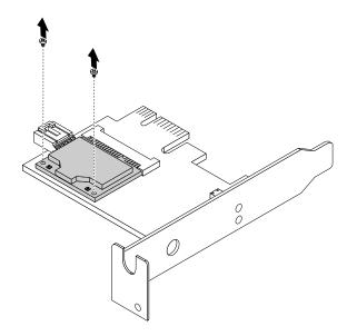
Figure 65. Removing the screws that secure the WiFi card module
