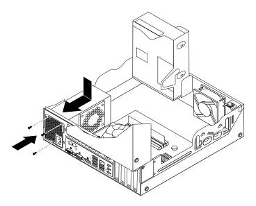
Figure 51. Installing the power supply assembly
