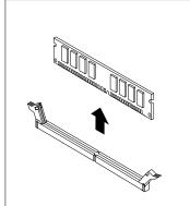
Figure 12. Removing a memory module
