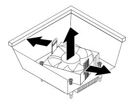
Figure 46. Removing the heat sink fan duct
