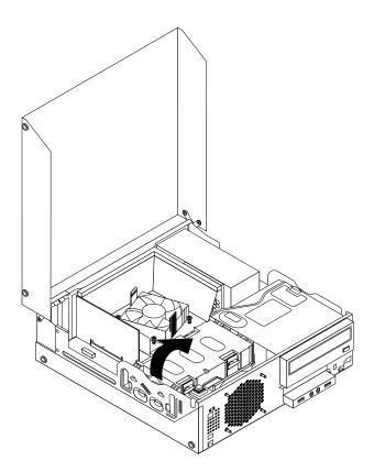
Figure 38. Removing the hard disk drive
