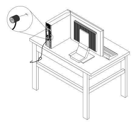
Figure 8. Integrated cable lock
