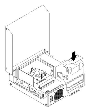
Figure 44. Installing a new optical drive
