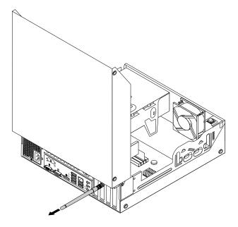
Figure 71. Removing the rear WiFi antenna
