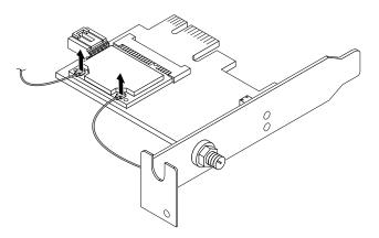
Figure 64. Removing the WiFi antenna cables
