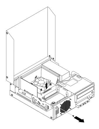
Figure 57. Removing the cover presence switch
