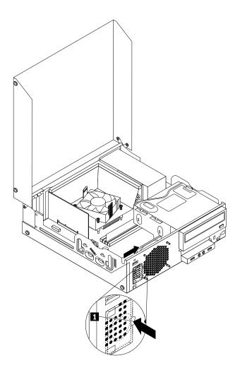
Figure 59. Removing the internal speaker
