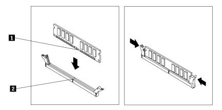
Figure 14. Installing a memory module
