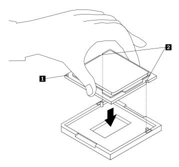
Figure 55. Installing the microprocessor
