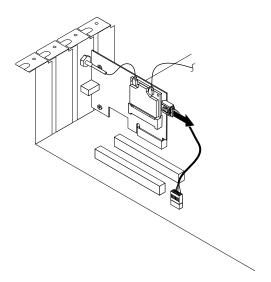
Figure 62. Disconnecting the Bluetooth cable
