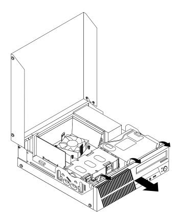
Figure 10. Removing the front bezel
