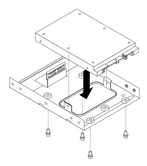
Figure 36. Installing the solid state disk into the adapter
