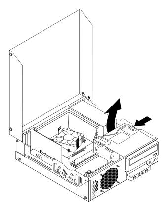
Figure 41. Pivoting the optical drive bay
