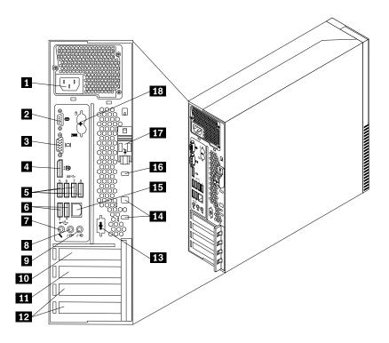
Figure 2. Rear connector locations
