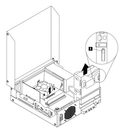
Figure 42. Removing the old optical drive
