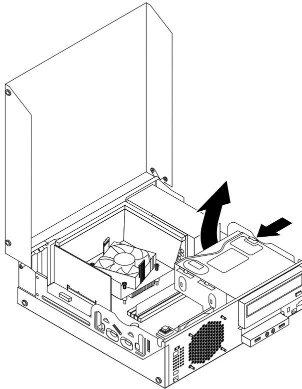
*Figure 41. Pivoting the optical drive bay*
