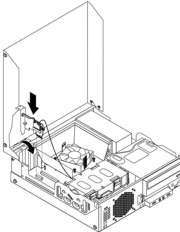
Figure 69. Installing the WiFi adapter card
