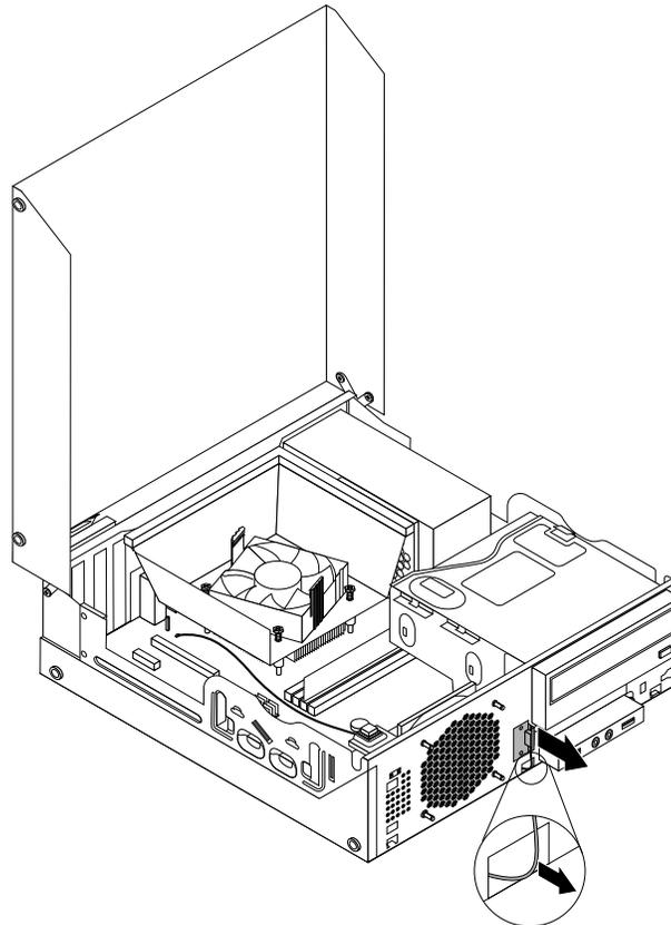
Figure 74. Removing the front WiFi antenna
