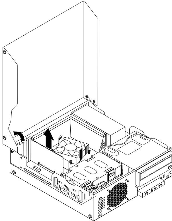
Figure 15. Removing a PCI card
