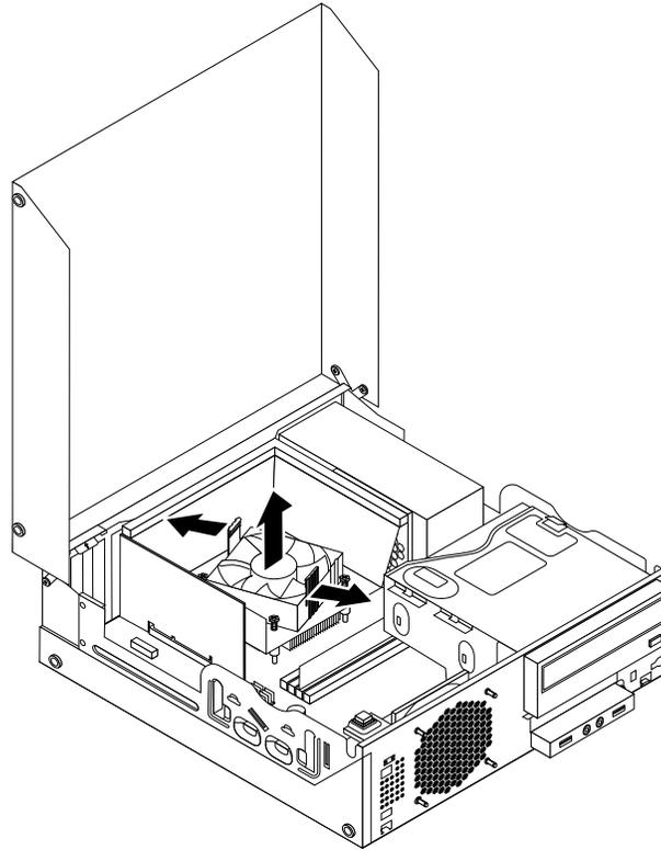
*Figure 48. Removing the heat sink fan duct*
