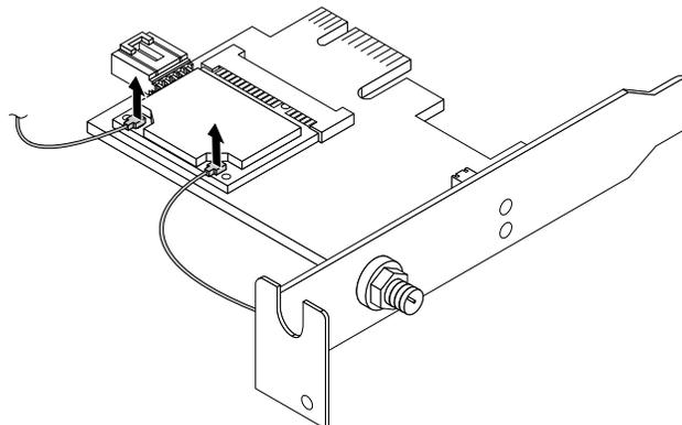
Figure 64. Removing the WiFi antenna cables
