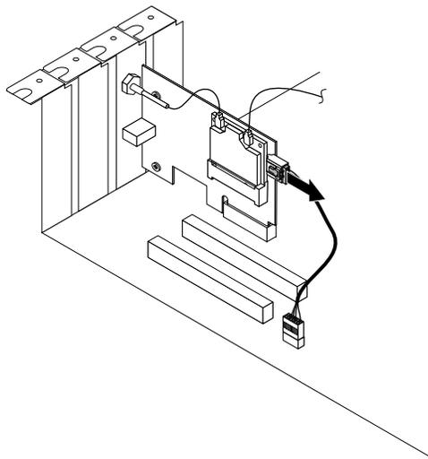
Figure 62. Disconnecting the Bluetooth cable
