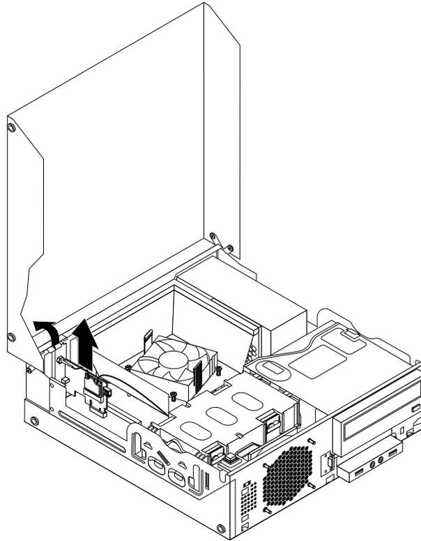
Figure 63. Removing the WiFi adapter card
