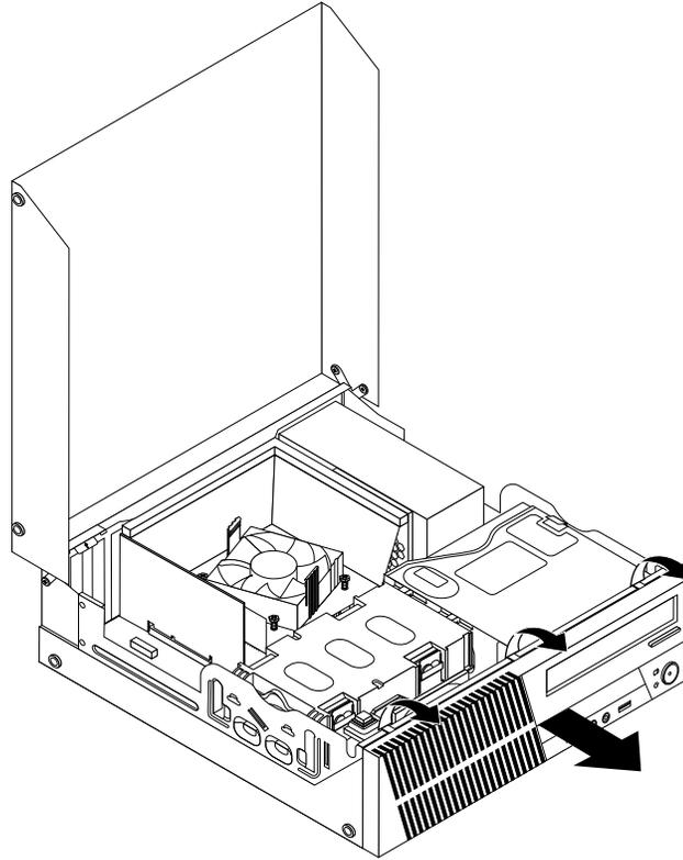
*Figure 10. Removing the front bezel*
