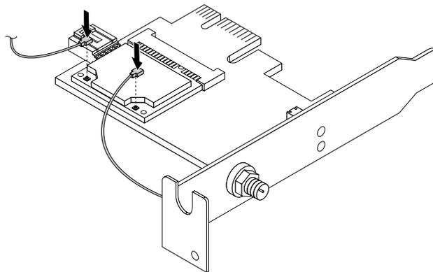
Figure 68. Connecting the WiFi antenna cables
