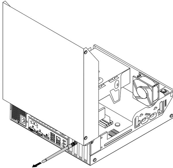
Figure 71. Removing the rear WiFi antenna
