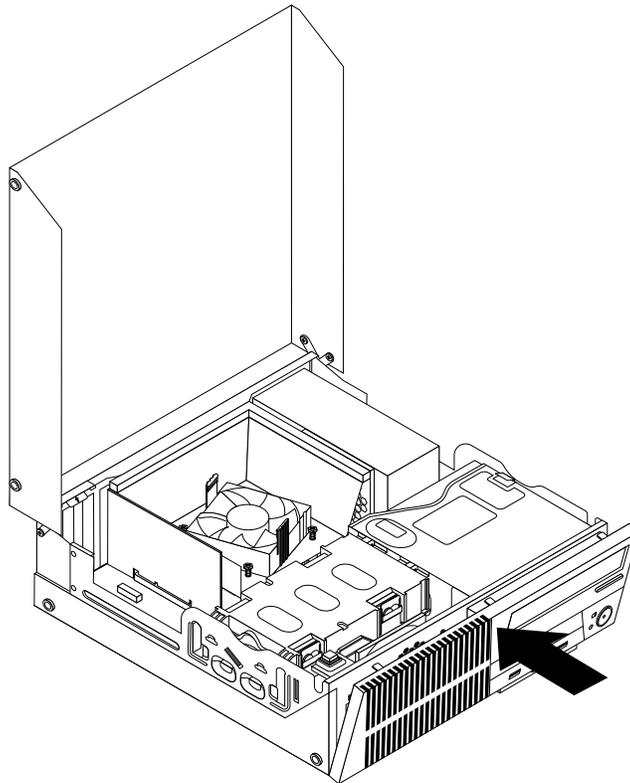
Figure 11. Reinstalling the front bezel
