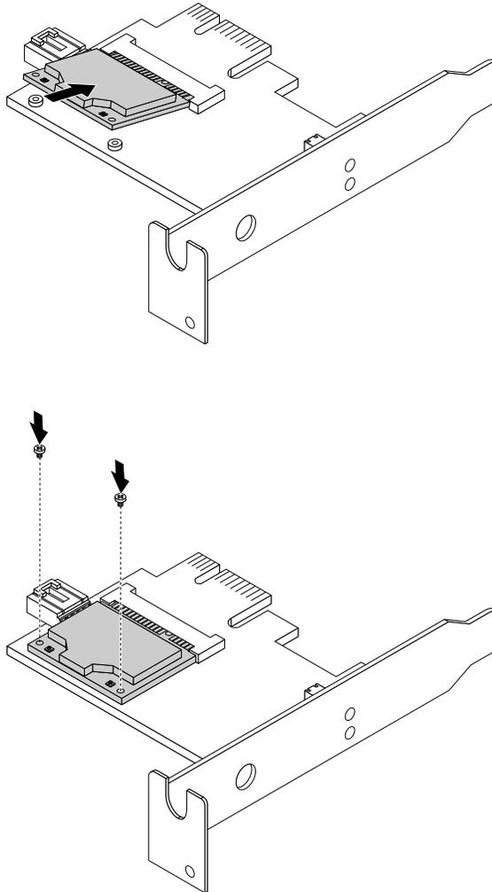
Figure 67. Installing the WiFi card module
