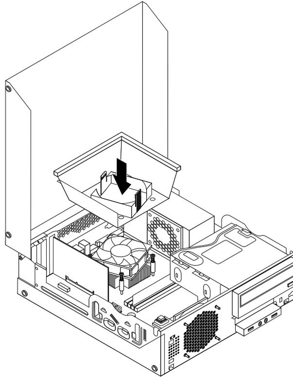
Figure 47. Installing the heat sink fan duct
