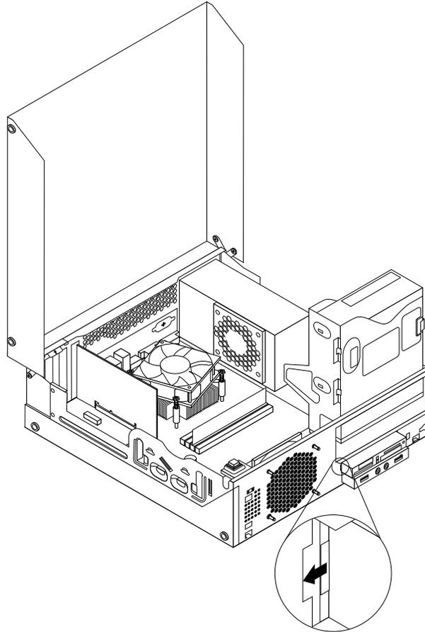
Figure 21. Installing the card reader
