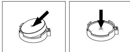
Figure 35. Installing a new battery
