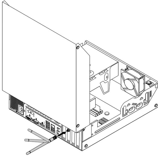
*Figure 70. Installing the rear WiFi antenna*
