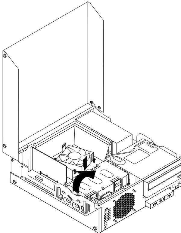
Figure 38. Removing the hard disk drive
