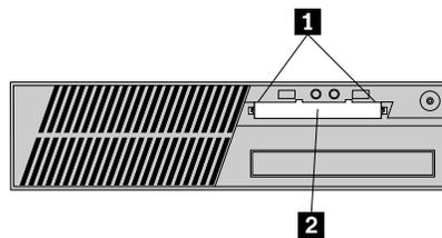
Figure 19. Removing the card reader cover
