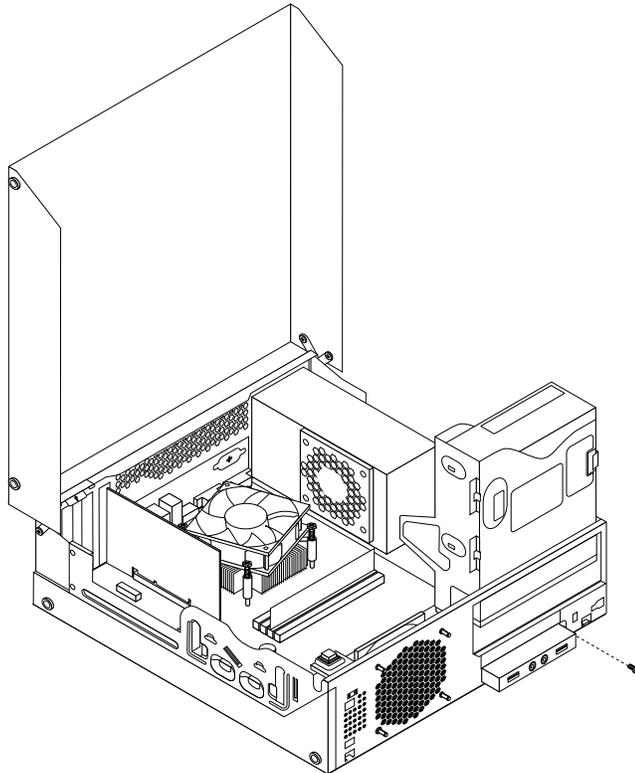
*Figure 61. Removing the front audio and USB assembly*
