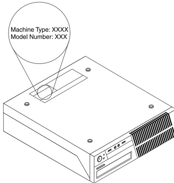
*Figure 7. Machine type and model label*
