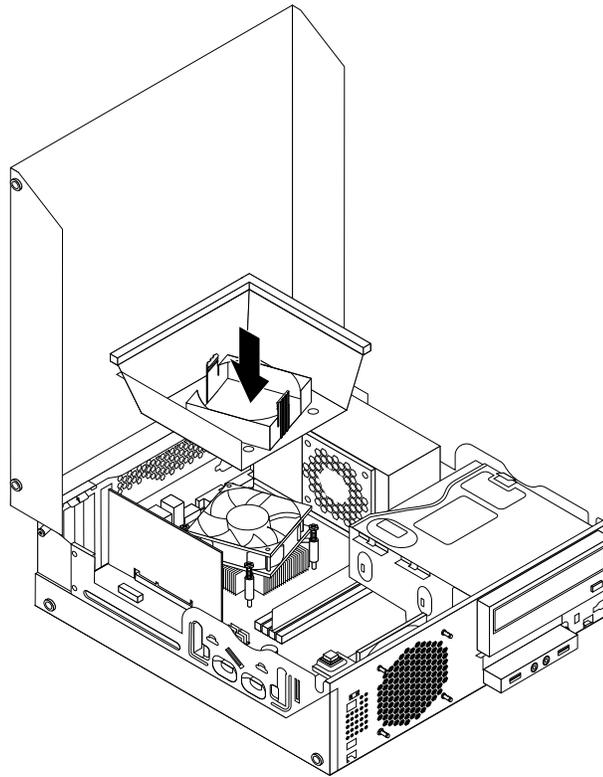
Figure 52. Installing the heat sink fan duct
