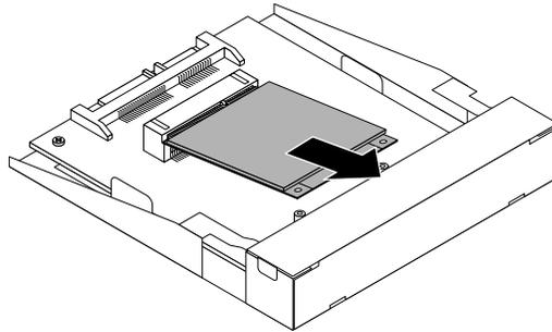
*Figure 29. Removing the mSATA solid state drive*
