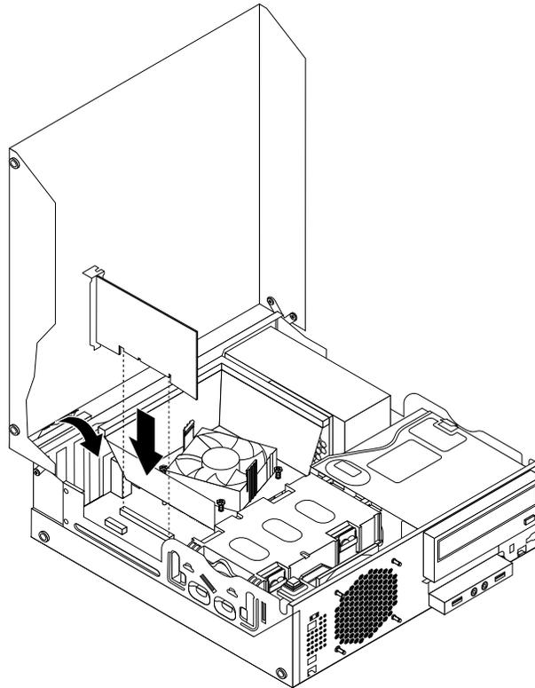
Figure 16. Installing the PCI card
