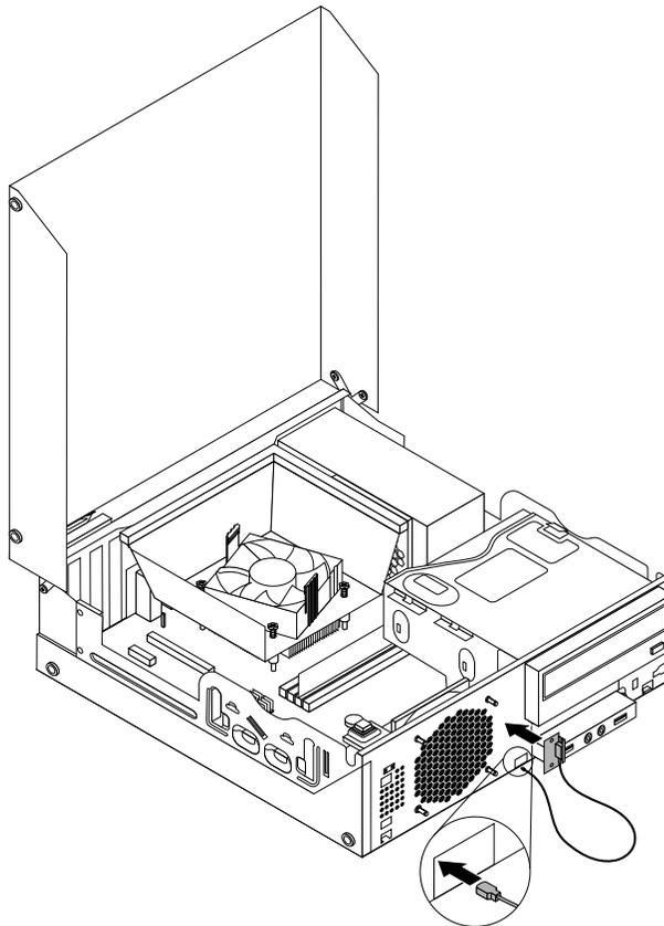
Figure 73. Installing the front WiFi antenna
