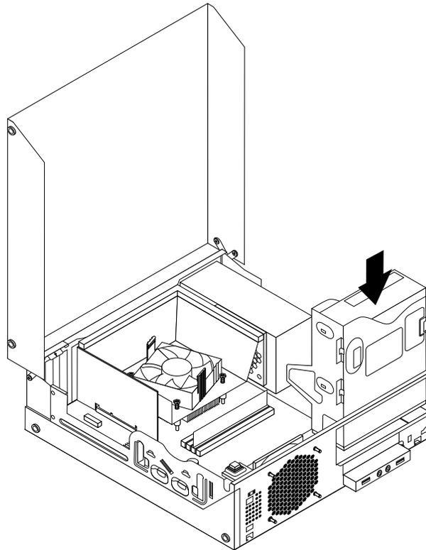
Figure 44. Installing a new optical drive
