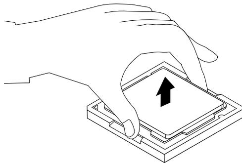
Figure 54. Removing the microprocessor
