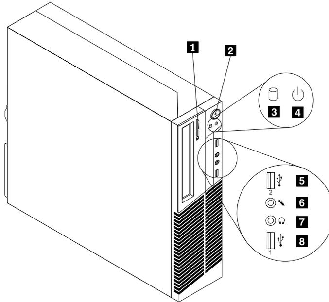
Figure 1. Front connector, control, and indicator locations
