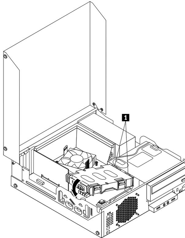
Figure 40. Installing the hard disk drive
