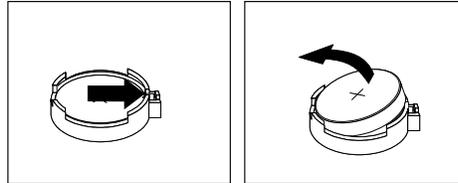
Figure 34. Removing the old battery
