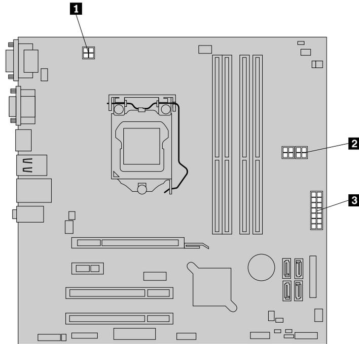
Figure 49. Power connectors on the system board
