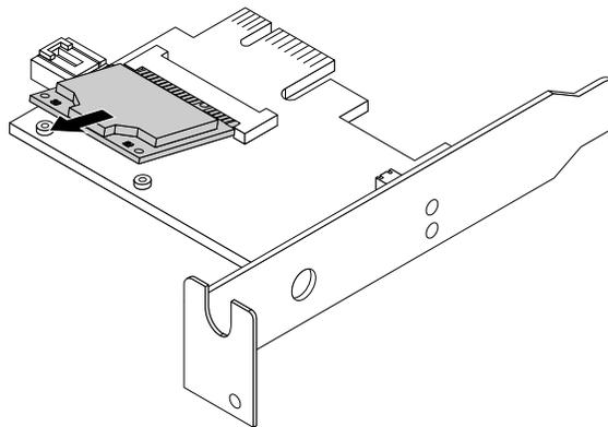
Figure 66. Removing the WiFi card module
