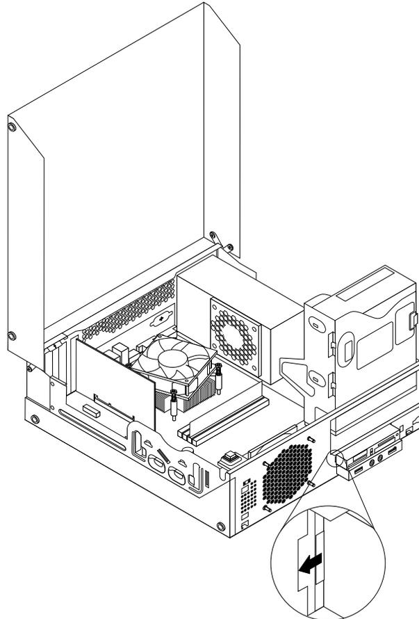
Figure 17. Installing the card reader
