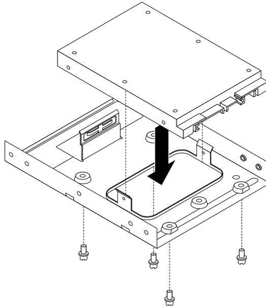
Figure 36. Installing the solid state disk into the adapter
