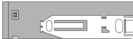
Figure 43. Installing the optical drive retainer
