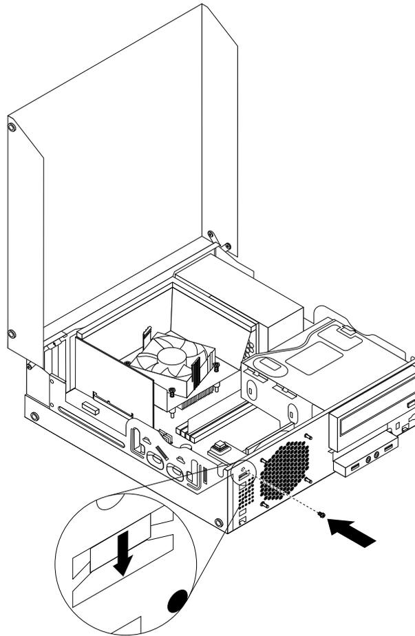
Figure 58. Installing the new cover presence switch
