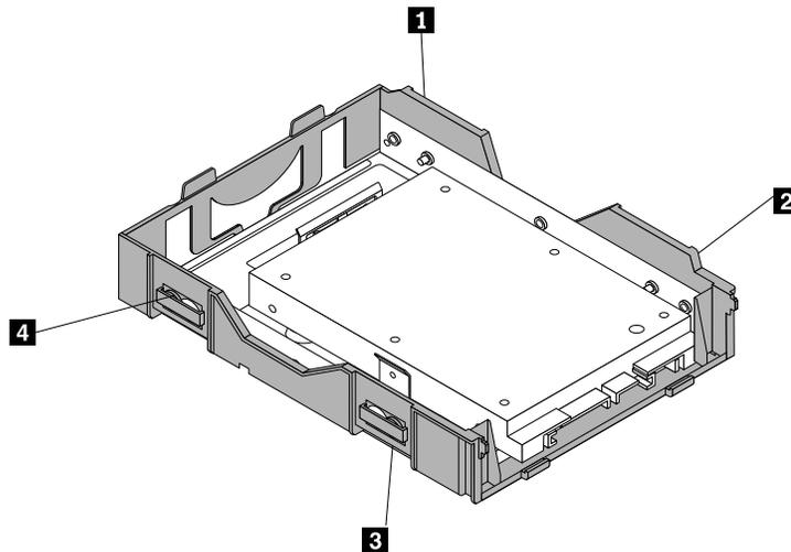
Figure 37. Installing the solid state disk with the adapter into the hard disk drive bracket
