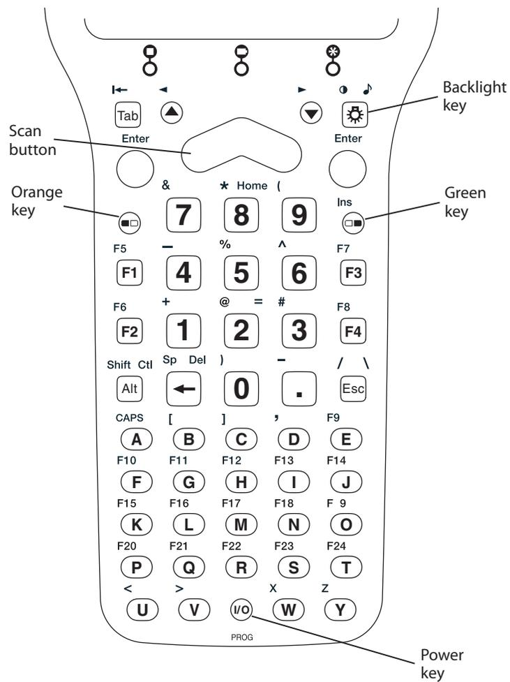
**52-key full alphanumeric keypad:** This keypad is designed for applications that enter mainly numeric data (0-9) and that may need to enter the entire alphabet. The keypad also provides function keys (F1-F24) and special characters, symbols, and functions by pressing color-coded key sequences.
