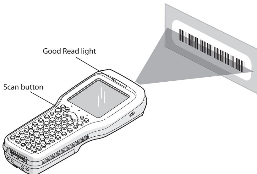
**Scanning:** Using the integrated laser scanner or 1D linear imager to scan a bar code label.
