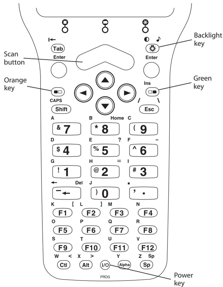
**42-key large numeric and function keypad:** This keypad is designed for applications that enter mainly numeric data (0-9) and that need dedicated function keys (F1- F12). This keypad also lets you enter the entire alphabet and special characters by pressing color-coded key sequences.
