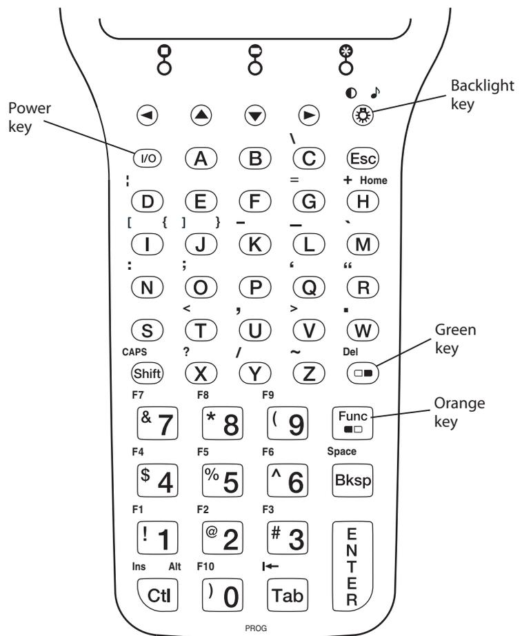
**50-key full alphanumeric keypad:** This keypad is designed for applications that enter mainly numeric data (0-9) and that may need to enter the entire alphabet. The keypad also provides shifted function keys (F1-F9) and special characters, symbols, and functions by pressing color-coded key sequences.
