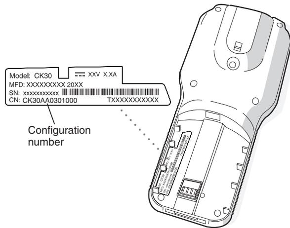
**Configuration Label:** The label in this illustration is for a CK30 Model A (CK30A).
