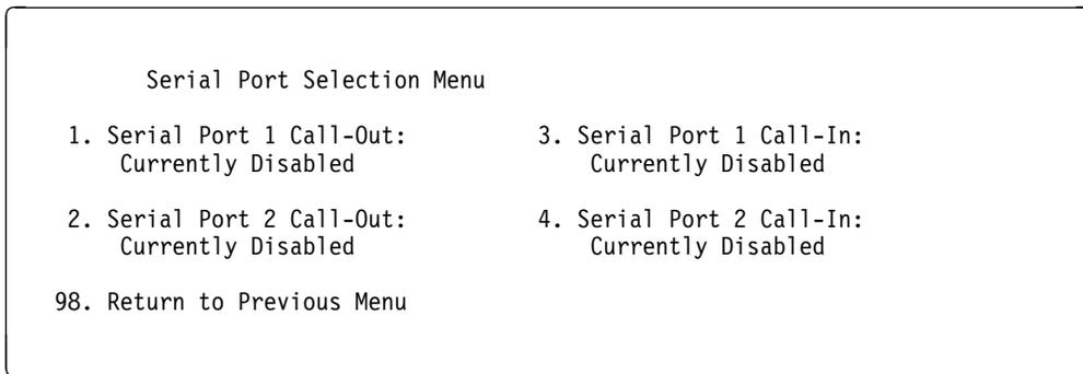
Call-in and ring indicate power-on cannot be enabled at the same time. If ring indicate power on is already enabled and you try to enable call-in, a message prompts you for confirmation. Refer to the message displayed on the screen.
