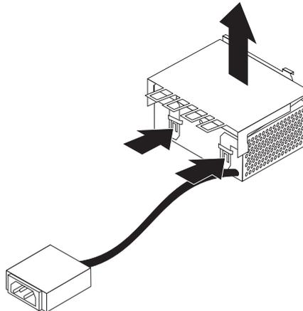
4. Lift out the power supply and plug.
