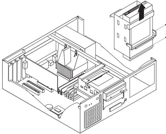
2. Remove the two screws that hold the CD-ROM drive in place. Lift the CD-ROM drive out of the cage.
