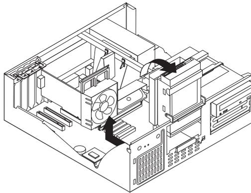
4. Lift the fan/speaker bracket back and out.
