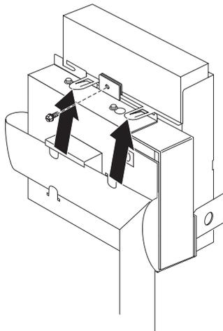
4. Remove the HD cable from the drive and from the bottom of the drive cage. Note the placement of the cable under the three tabs.
