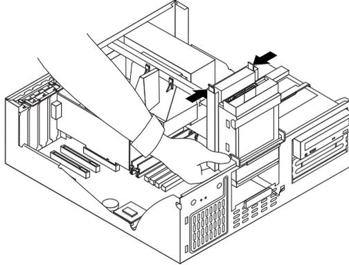
3. When replacing the drive cage into its horizontal position, be sure place the cage latch back to its regular horizontal position. This is necessary so that the machine cover will fit properly.
