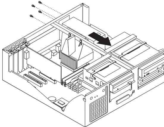
2. The power supply is attached to the base of the chassis by a latch on the front. Slide the power supply forward to dislatch it from the chassis.
