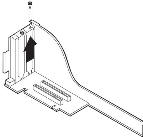
3. Remove the screw and adapter slot cover for the adapter slot into which you are installing the adapter.
