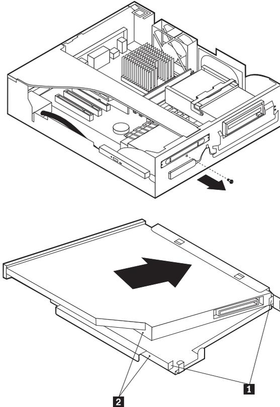
4. Install the slimline CD-ROM drive into the drive bay bracket, aligning the tabs on the bay bracket **1** with the rear of the slimline CD-ROM drive **2** and the tiny holes in the drive with the retaining pins in the drive bay bracket.
