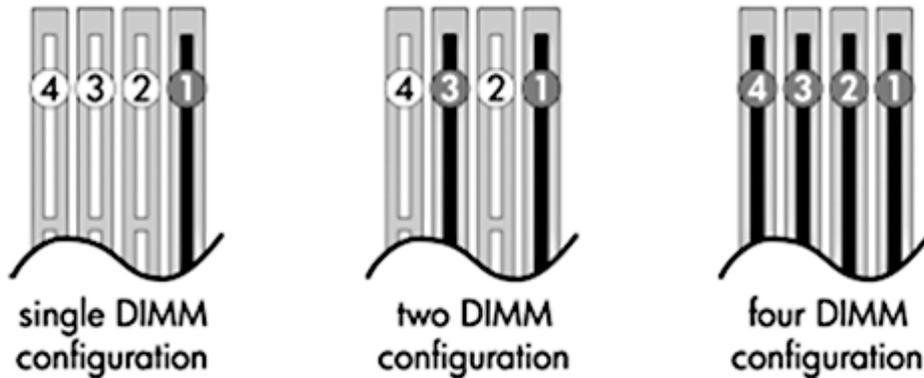
If only using 1 DIMM, install in socket 1. If using 2 DIMMs, install them in sockets 1 & 3. If using 4 DIMMs, install them in all sockets.
