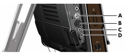
If you are using S-Video, connect audio cable from your set-top box to the Audio line in (C) connector on the back of the computer. Use with a Y cable to combine RCA left and right channels (white and red).
