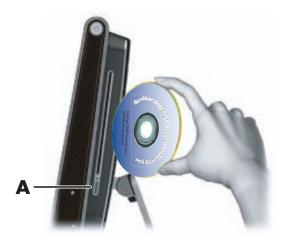
To eject a disc, make sure the power is turned on and then press the eject button (**A**) on the side of the disc drive. You can also tap the **Windows Vista start button** (**b**), tap **Computer**, press and hold (or with the mouse, right-click) the CD drive, and then tap **Eject**.
