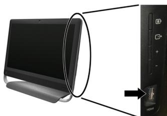
When a device is plugged into the HDMI port, the volume on the computer is muted. Pressing the +/- buttons on the side panel does not change the volume of the computer.
