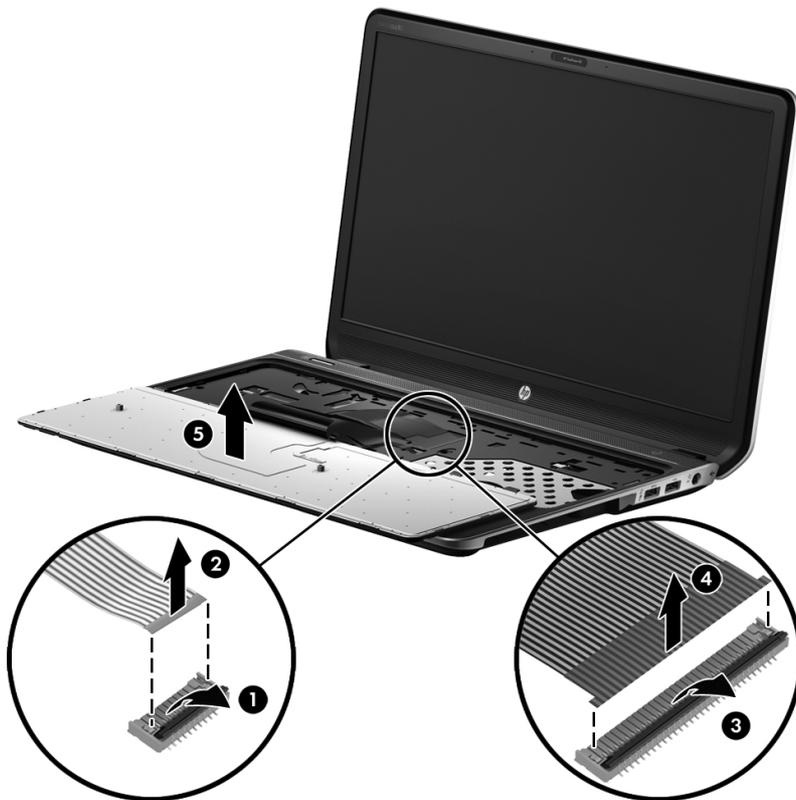
Reverse this procedure to install the keyboard.
