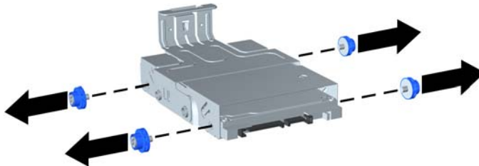
Figure 2-16 Removing the Guide Screws
