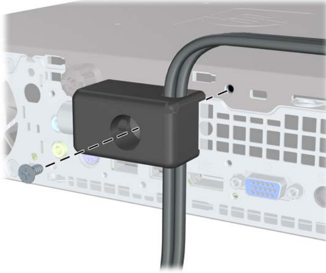
Figure C-6 Attaching the Lock to the Chassis
