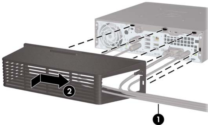
Figure 2-21 Installing a Port Cover
