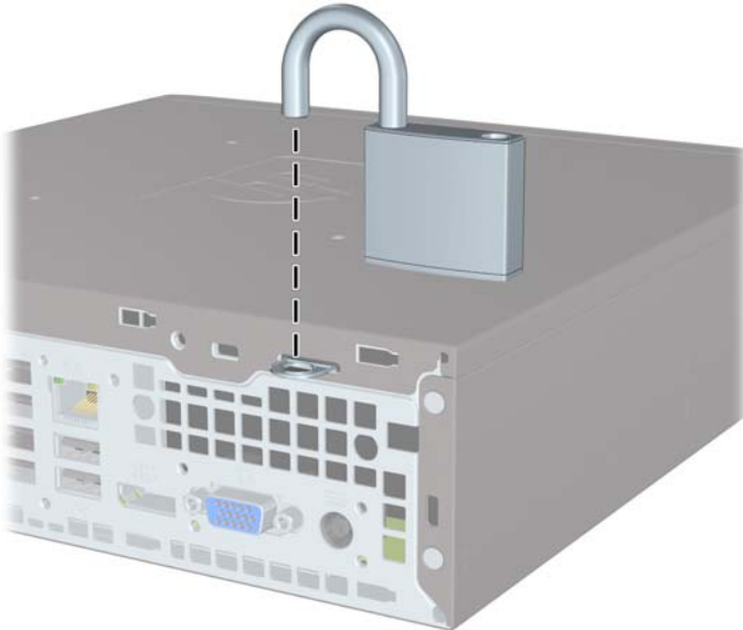
Figure C-3 Installing a Padlock
