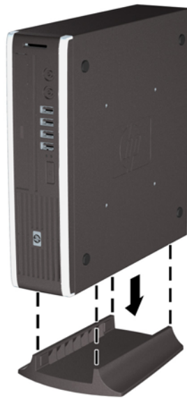
Figure 2-7 Placing the Computer on the Stand
