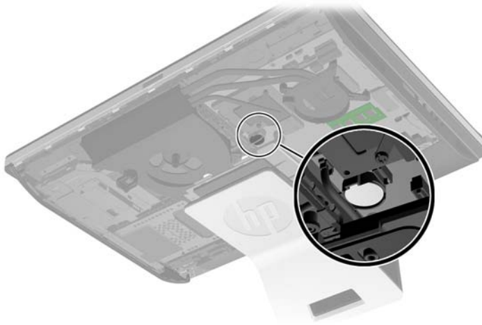
Figure 7-32 Locating the battery
