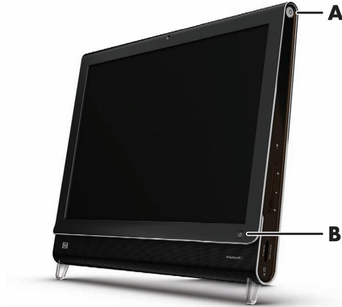
You can also turn on the HP TouchSmart PC or put it into Sleep mode by pressing the Power/Sleep button on the keyboard or the remote control. A remote control is included with select models only.
