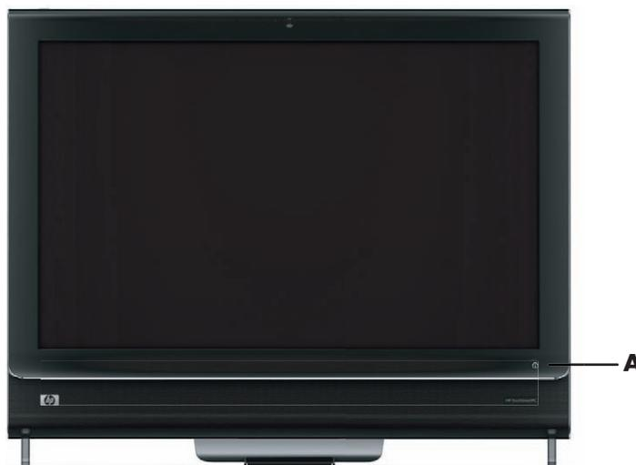
To open the HP TouchSmart software, just press the HP TouchSmart button (**A**) on the lower-right side of the HP TouchSmart PC.
