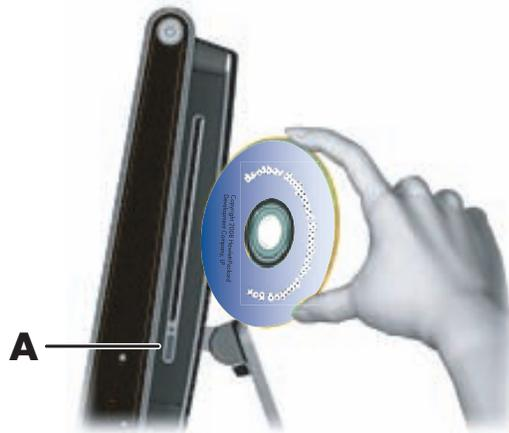
To eject a disc, make sure the power is turned on and then press the eject button (**A**) on the side of the disc drive. You can also tap the **Windows Vista start button**
