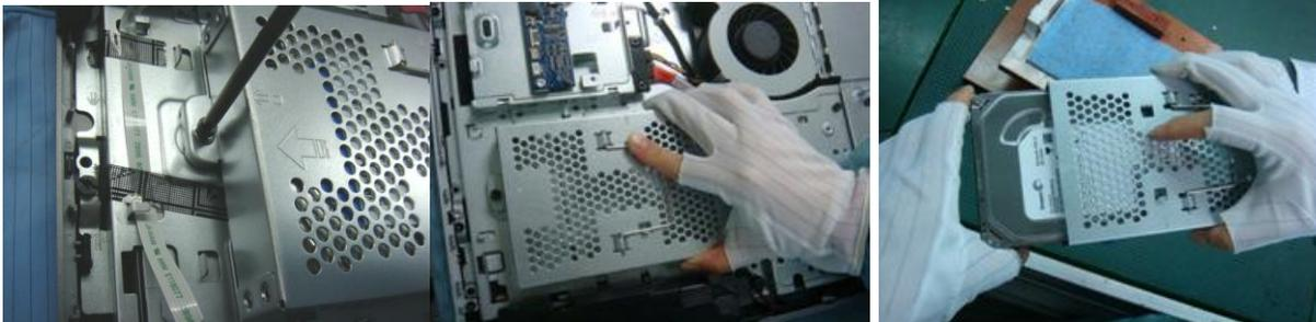
Remove one screw and push ODD forward to slide from ODD cage.
