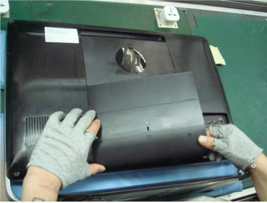
2) Disassemble hinge cover and rear cover.
