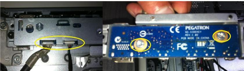
13) Disassemble Converter board
