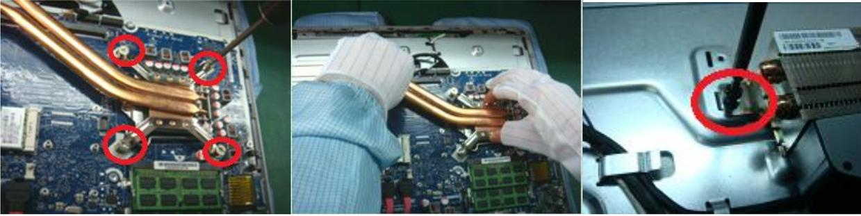
10) Disassemble MXM thermal module and remove the graphic card (with Graphic card module)
