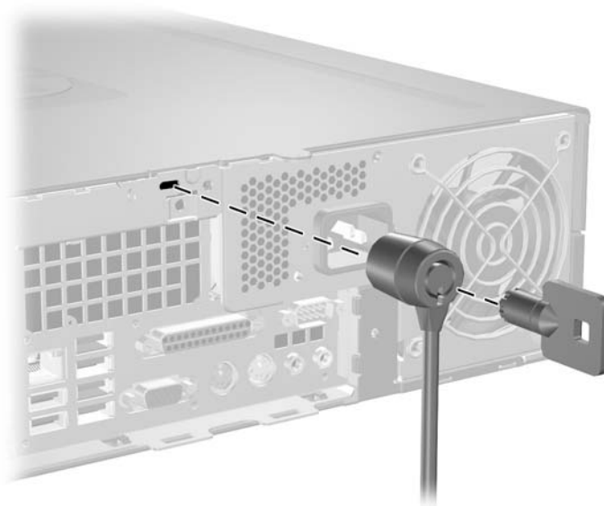
Installing a Cable Lock
