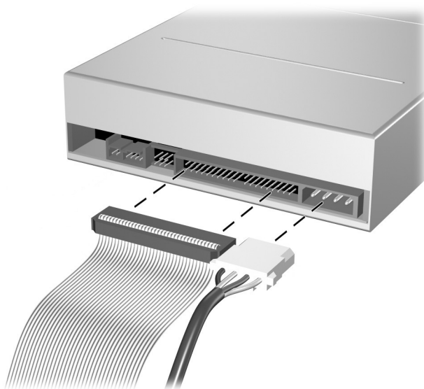
Reconnecting the Optical Drive Cables
