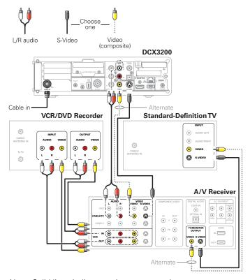
Note: Solid lines indicate optimum connections.
