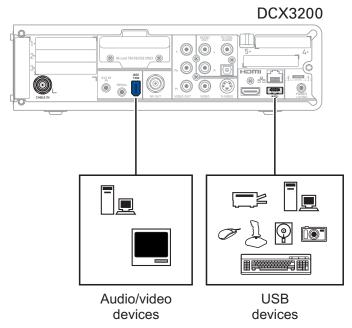
Note: Do not attempt to connect data devices without contacting your service provider. Advanced data features require the proper application and network infrastructure to operate.
