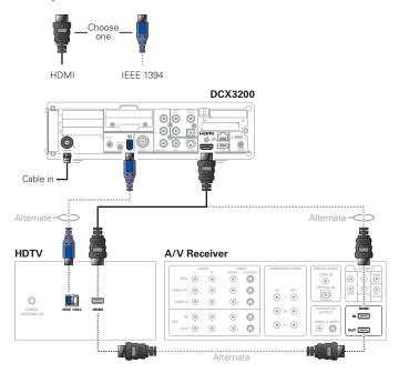
Note: Only (1) HDTV video/audio connection needs to be made to an HDTV.
