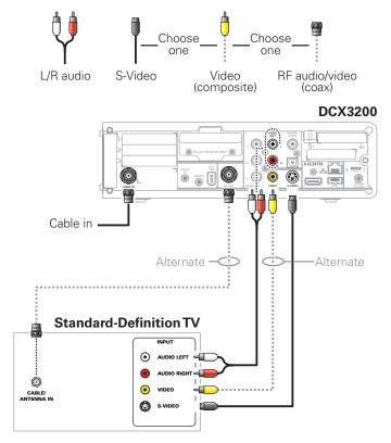
Note: S-Video and Composite video require separate audio connections.
