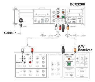
Note: Only (1) audio connection needs to be made to an A/V Receiver.
