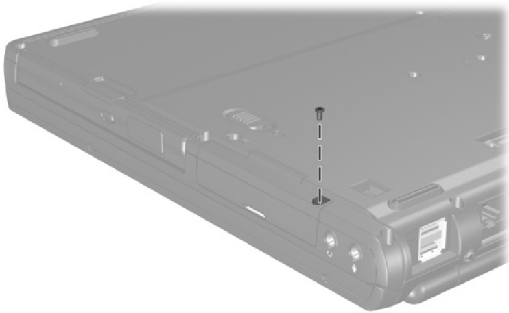
Phillips PM2.0x4.0 Hard Drive Cover Screw Location
