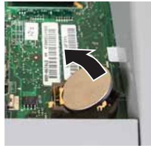
Carefully pry with screwdriver here
