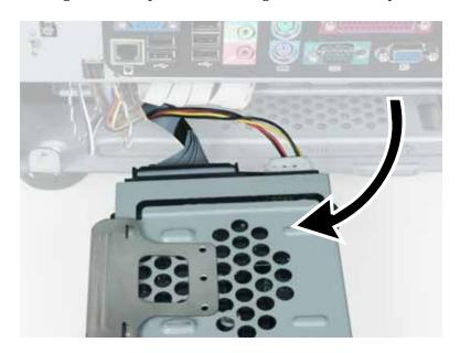
**7** Disconnect the drive cable and power cable from the hard drive.
