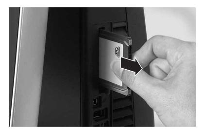
**3** Eject the PC Card by pressing the eject button again.
