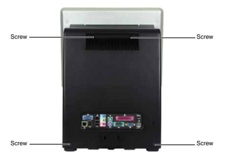
**5** With your hands positioned on each side of the case, swing the back panel up and away from the case and set the panel aside.
