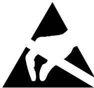
Boards with electrostatic sensitive devices (ESD) are identifiable by the label shown.
