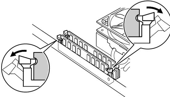
**6 Insert the slot into the memory.**
