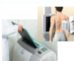
Images recorded on the Imaging Plate (IP) are read with an image reader. IPs can be repeatedly used since images can be erased.
