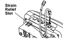
3. Plug the modular cord's other end into a modular telephone line jack.
