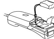
3. Insert the new battery pack's connector into the socket in the compartment, place the battery pack into the compartment, and refasten the retainer strap.
