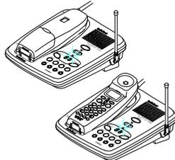
Recharge the battery pack when **RECHARGE NOW** appears and
