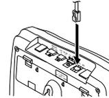
3. Insert the supplied AC adapter's barrel plug into the DC IN 9V jack.
