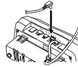
5. Route the adapter's cord through the strain relief slot on the bottom of the bracket.
