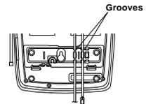
6. Align the bracket's keyhole slots with the mounting screws and slide the base downward to secure it.
