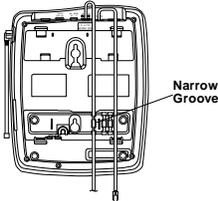
5. Plug the modular cord's other end into the wall plate jack, then align the bracket's keyhole slots with the wall plate studs and slide the base downward to secure it.
