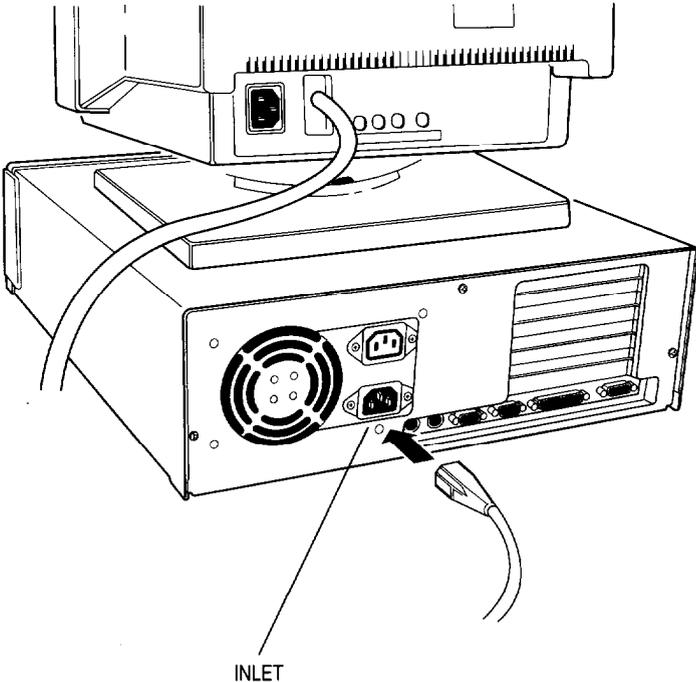
2. Plug the other end of the power cord into an appropriate grounded (earthed) electrical outlet.
