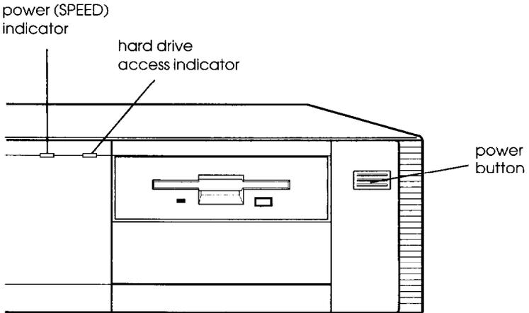
The power indicator on the left side of the front panel lights up. After a few seconds, the screen displays a count of the system memory, and then the computer performs a power-on diagnostics routine to make sure everything is working correctly.
