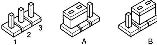
In the off position, a three pin jumper sits on only one of the end pins. To move a jumper from one position to the other, use needle-nose pliers or tweezers to pull it off its pins and gently move it to the desired position.
