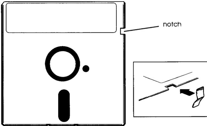
To remove the write protection, peel off the write-protect tab.
