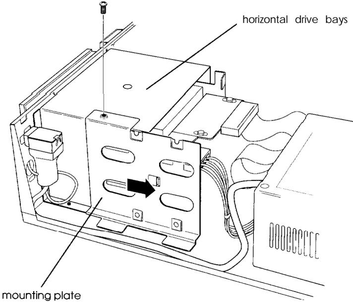
2. Turn the hard disk drive so the components face up and the connectors face left. Then place the mounting plate on the hard disk drive and align the four holes in the plate with the four holes in the drive, as shown below.
