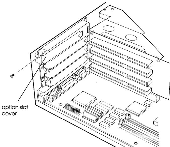
2. Slide out the slot cover and set it aside. (Store the slot cover in a safe place in case you remove the option card later.)
