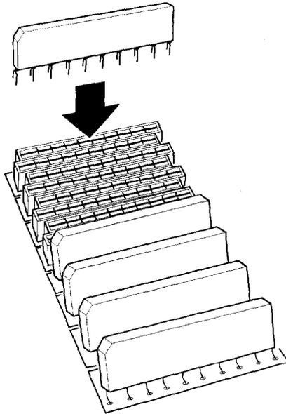
5. Gently press the chip halfway into the socket (to make sure it is correctly aligned). If the chip does not go in smoothly, remove it and try again.
