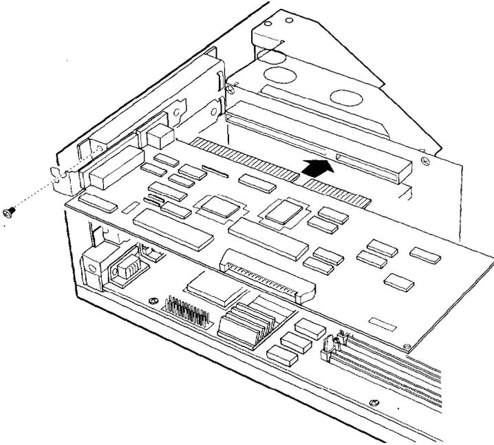
Once the connectors reach the slot, push the card in firmly (but carefully) to insert it fully. You should feel the card fit into place. If it does not go in smoothly, do not force it; pull the card all the way out and try again.
