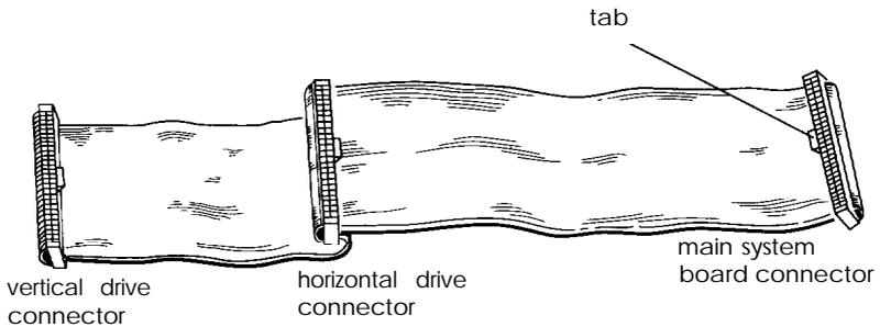
3. Select the connector on the end of the longest part of the cable (the main system board connector). Notice the small tab in the middle of the cable connector, as shown in the illustration above. Align the connector so that the tab aligns with the notch, as shown below. (The option card connector board and diskette drive ribbon cable are removed from the illustration for clarity.)
