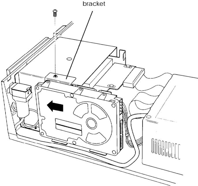
6. Secure the mounting plate with the screw, as shown above.
