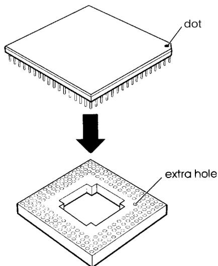
6. Make sure the pins in the processor chip are directly over the holes in the socket. Then gently push the processor straight into the socket, pressing evenly on all sides.
