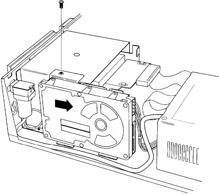
3. Remove the four screws securing the mounting plate to the hard disk drive. You can store the mounting plate and its screw or replace it in the computer and secure it with the screw.
