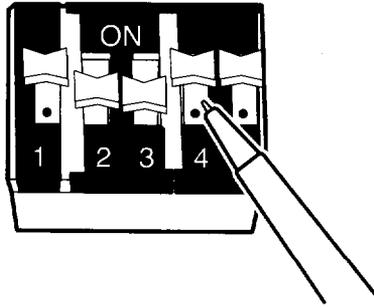
3. Depending on which DIP switch you change, you may also need to run SETUP. For example, if you set DIP switch 4 to ON to enable password security, you then need to enter your password using **Set Password options** in SETUP. See Chapter 2 for instructions.
