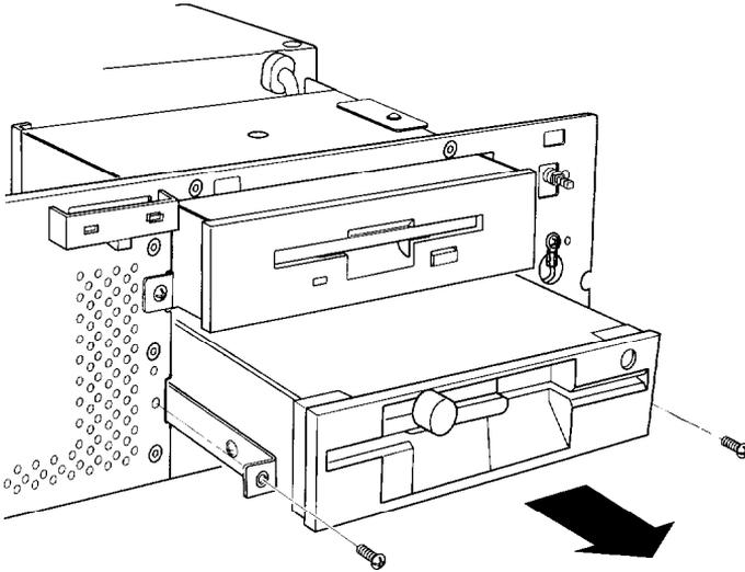
3. If you are leaving the drive bay empty, replace the metal drive bay cover and two retaining screws, as shown below.
