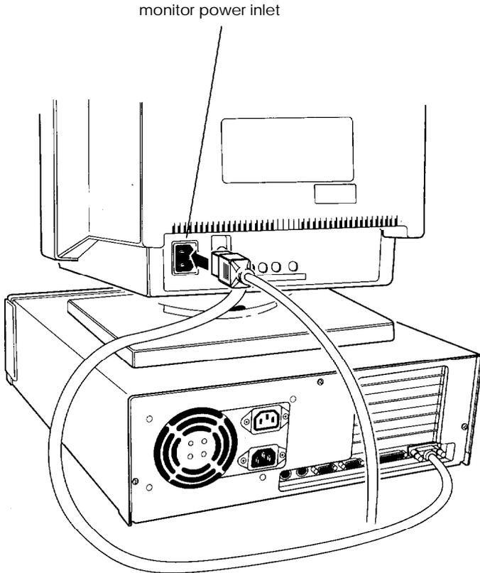
6. Plug the other end of the power cord into an appropriate grounded electrical outlet or, if the cord has the correct type of plug, into the power outlet on the back of the computer.
