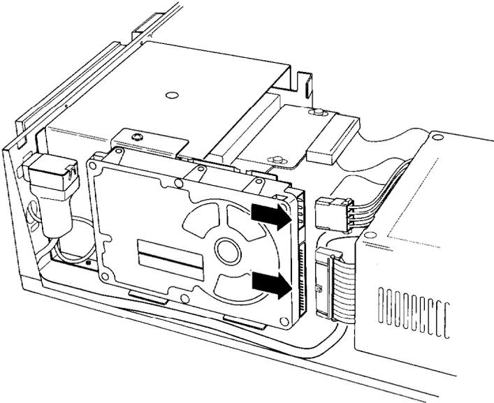
2. Remove the retaining screw securing the hard disk drive and mounting plate to the horizontal drive bays. Then slide the hard disk drive and mounting plate in the direction of the arrow, shown in the following illustration, and lift them out of the computer.
