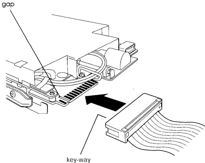
Make sure the cable connector fits properly onto the drive connector and push it into place. Be careful to align the connector correctly; otherwise, you could severely damage your drive when you push it in. Go to step 3.
