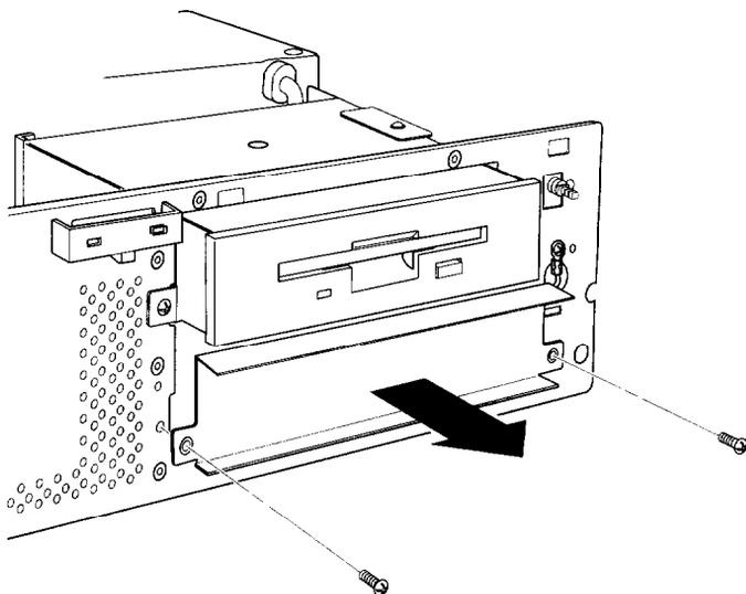
4. If you are installing a 5.25-inch diskette drive, hold it so that the diskette release latch is above the diskette slot. If you are installing a 3.5-inch diskette drive or a 5.25-inch dual drive, hold it so that the diskette release button(s) are on the right and the drive light is on the left.
