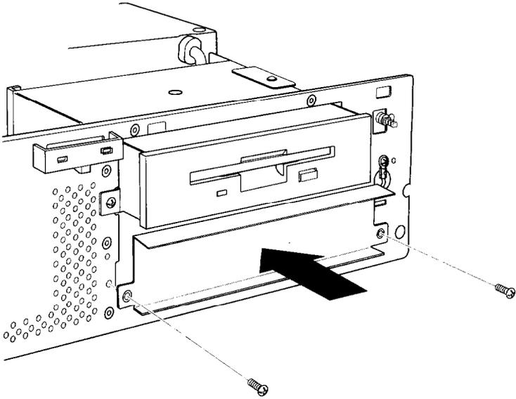
4. If you are replacing the drive you removed with another drive, remove the guiderails and screws from the drive and use them to install the other drive as described in “Installing a Drive in a Horizontal Bay” on page 5-16.
