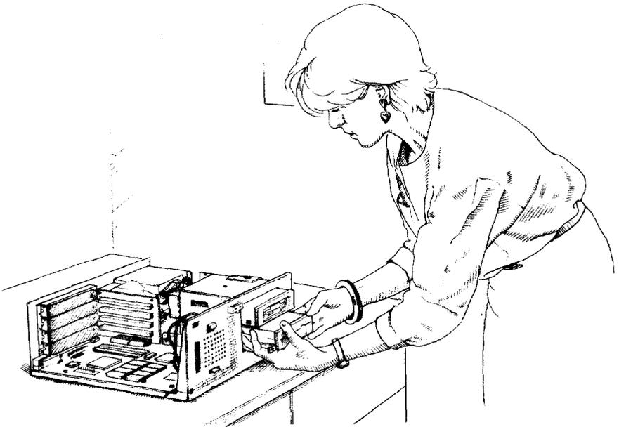
Your computer can hold up to three drives in two horizontal drive bays and one vertical drive bay.
