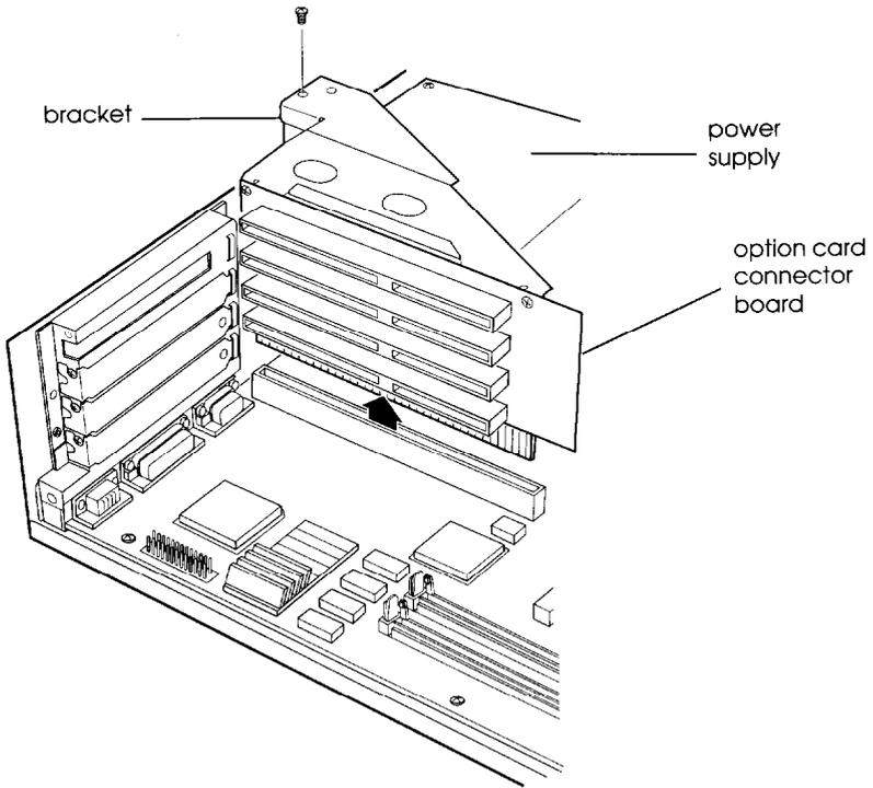
3. Pull the board straight up and out of its socket and set it aside.
