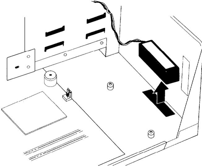
4. Remove the new battery from its package and position it so the Velcro faces down and the cable faces the power supply. Then push it down onto the bottom of the case.
