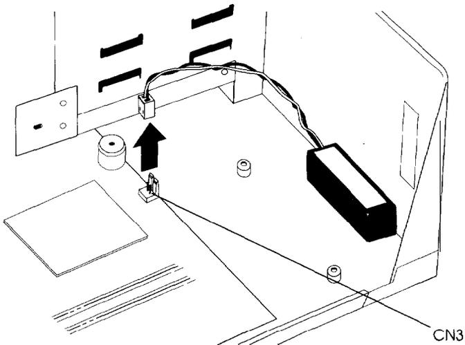
3. The battery is attached to the computer base with Velcro.<sup>®</sup> To remove it, pull it up from the bottom of the computer case, as shown in the following illustration. Then set it aside.
