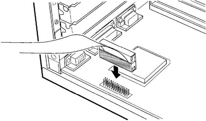
3. Connect the other end of the cable to the appropriate interface on the adapter card. (Check your graphics card manual for instructions.)
