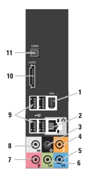
5 Connector — Connects to a microphone for voice or audio input into a sound or telephony program.
