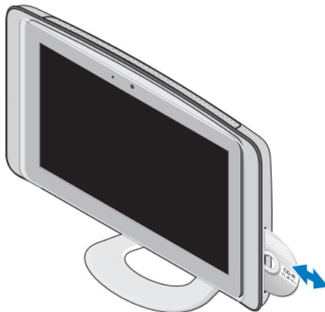
Insert the disc, with the label facing outwards and gently push the disc into the slot. The drive will automatically pull the disc in and begin reading its content. To eject a disc from the drive, gently touch the eject control.
