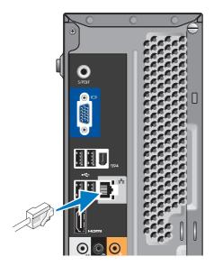
A network connection is not required to complete your computer setup, but if you have an existing network or Internet connection that uses a cable connection (such as a home cable modem or Ethernet jack), you can connect it now. Use only an Ethernet cable (RJ45 connector). Do not plug a telephone cable (RJ11 connector) into the network connector.
