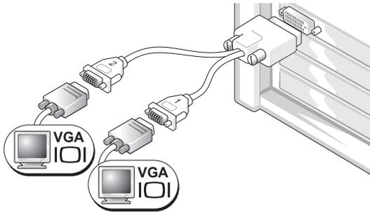
Use the appropriate Y cable when your graphics card has a single connector and you want to connect your computer to one or two VGA monitors.
