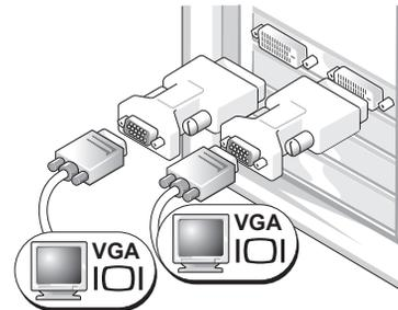
Use two VGA adapters to connect two VGA monitors to the DVI connectors on your computer.
