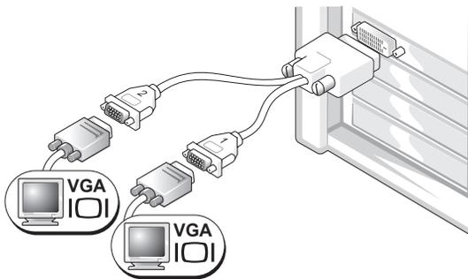
Use the appropriate Y cable when your graphics card has a single connector and you want to connect your computer to one or two VGA monitors.
