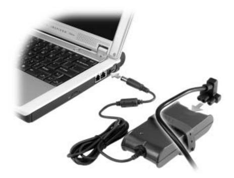
The AC adapter converts AC power to the DC power required by the computer. You can connect the AC adapter with your computer turned either on or off.
