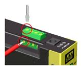
2. Screw the terminal and make sure power wire is fixed securely.
