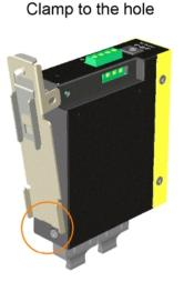
Screw the bracket on the device
