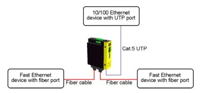
The following figure illustrates another example which deploys multiple fiber cables to connect other Ethernet devices in a daisy-chain method.
