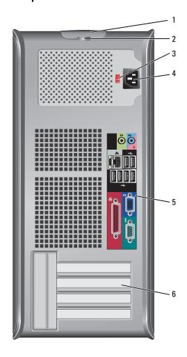
1 cover-release latch This latch allows you to open the computer cover.
