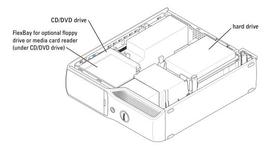
Connect CD/DVD drives to the connector labeled "IDE" on the system board. Serial ATA hard drives should be connected to the connectors labeled "SATA0" or "SATA2" on the system board.
