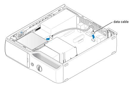
**6** Pull up on the drive release latch and slide the media card reader towards the back of the computer. Then, lift up to remove the drive from the computer.
