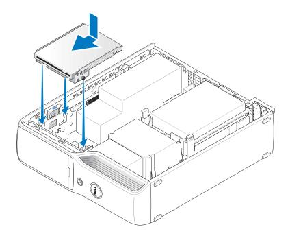
**5** Attach the power and data cables to the floppy drive.
