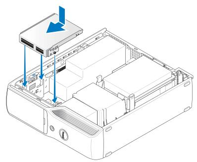
**6** Reconnect the data cable on the back of the media card reader to the front-panel connector on the system board.
