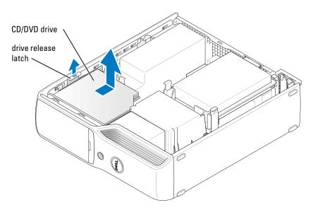
Disconnect the power and CD/DVD drive cables from the back of the drive.
