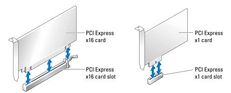
If you are installing or replacing a PCI Express card, follow the procedures in the next section. If you are removing but not replacing a card, see "Removing a PCI Express Card" on page 70. If you are replacing a card, remove the current driver for the card from the operating system.
