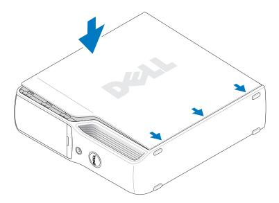
**c** Snap the cover into place by pulling back on the cover release latch, and then releasing the latch when the cover is properly seated.
