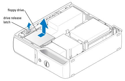
**6** Disconnect the power and data cables from the back of the floppy drive.
