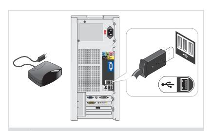
Connect the sensor for the optional remote control
