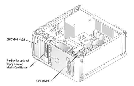
Connect CD/DVD drives to the connector labeled "IDE" on the system board. Serial ATA hard drives should be connected to the connectors labeled "SATA0" or "SATA2" on the system board.
