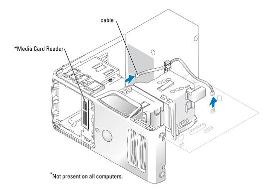
**5** Disconnect the USB cable on the back of the Media Card Reader to the front panel USB connector on the system board (see page 61) and route the cable through the clip on the shroud.
