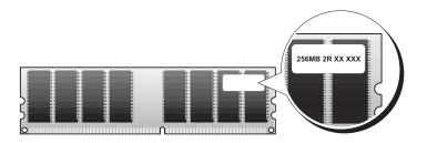
**NOTE:** Always install DDR2 memory modules in the order indicated on the system board.
