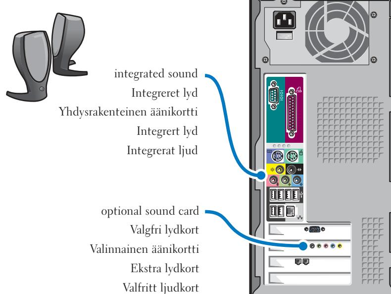
If your integrated sound connectors are covered by a cap, connect your speakers to the optional sound card connectors. Do not remove the cap.
