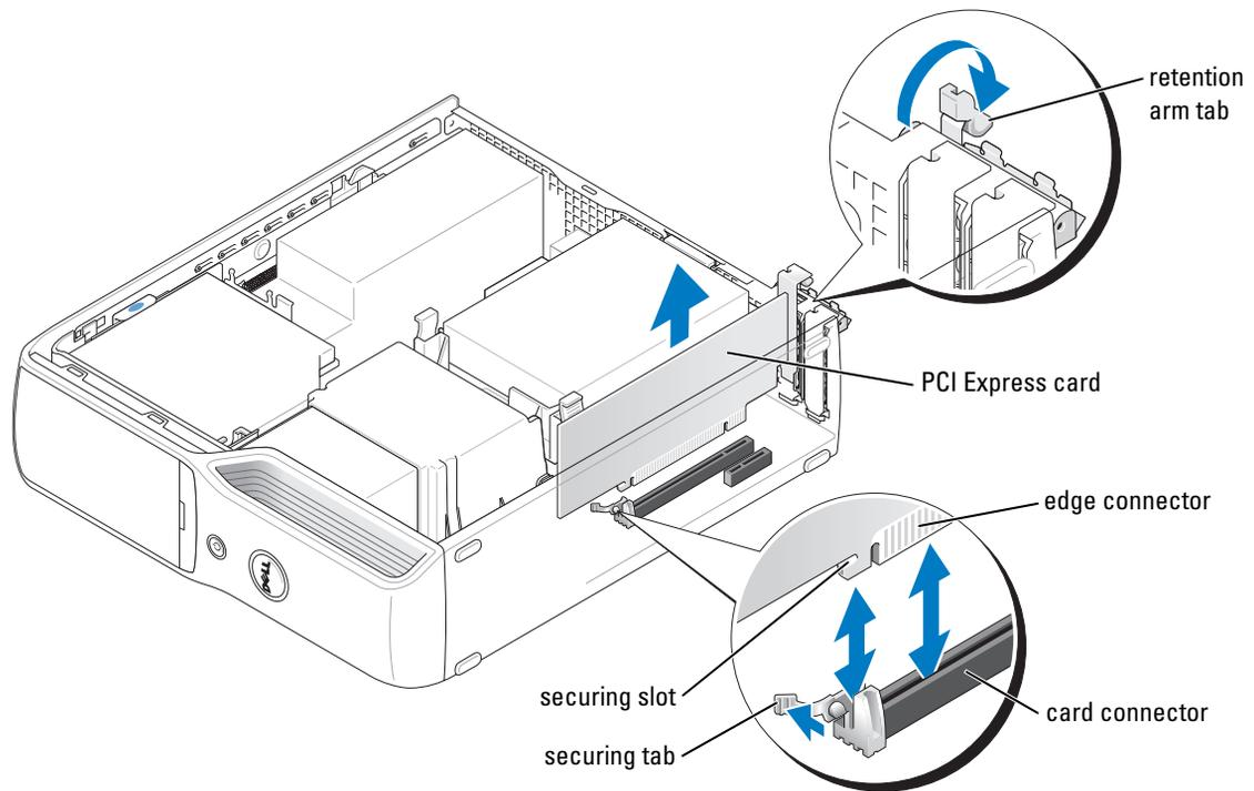
**3** If you are installing a new card, remove the filler bracket to create a card-slot opening. Then continue with step 5.
