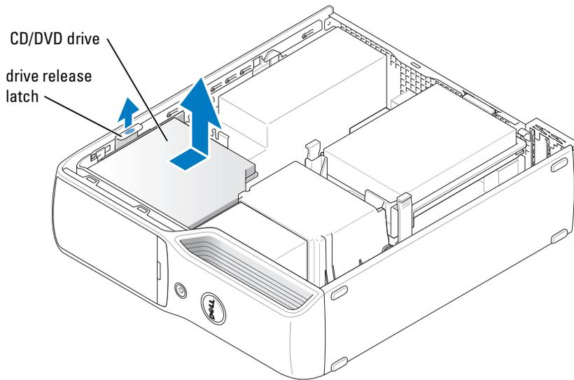
**NOTE:** The interface cable is held in place by the metal drive bracket and does not need to be removed from the drive.
