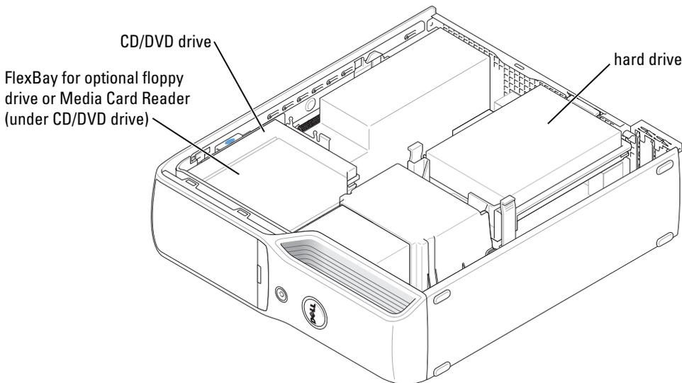
Connect a CD or DVD drive to the connector labeled "IDE\_OPT" on the system board. A serial ATA hard drive should be connected to the connector labeled "SATA0" on the system board.
