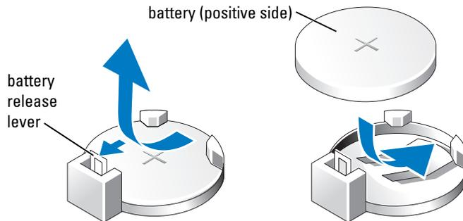
**➡ NOTICE:** To avoid damage to the battery connector, you must firmly support the connector while installing or removing a battery.
