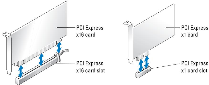
If you are installing or replacing a PCI Express card, follow the procedures in the next section. If you are removing but not replacing a card, see "Removing a PCI Express Card" on page 72.
