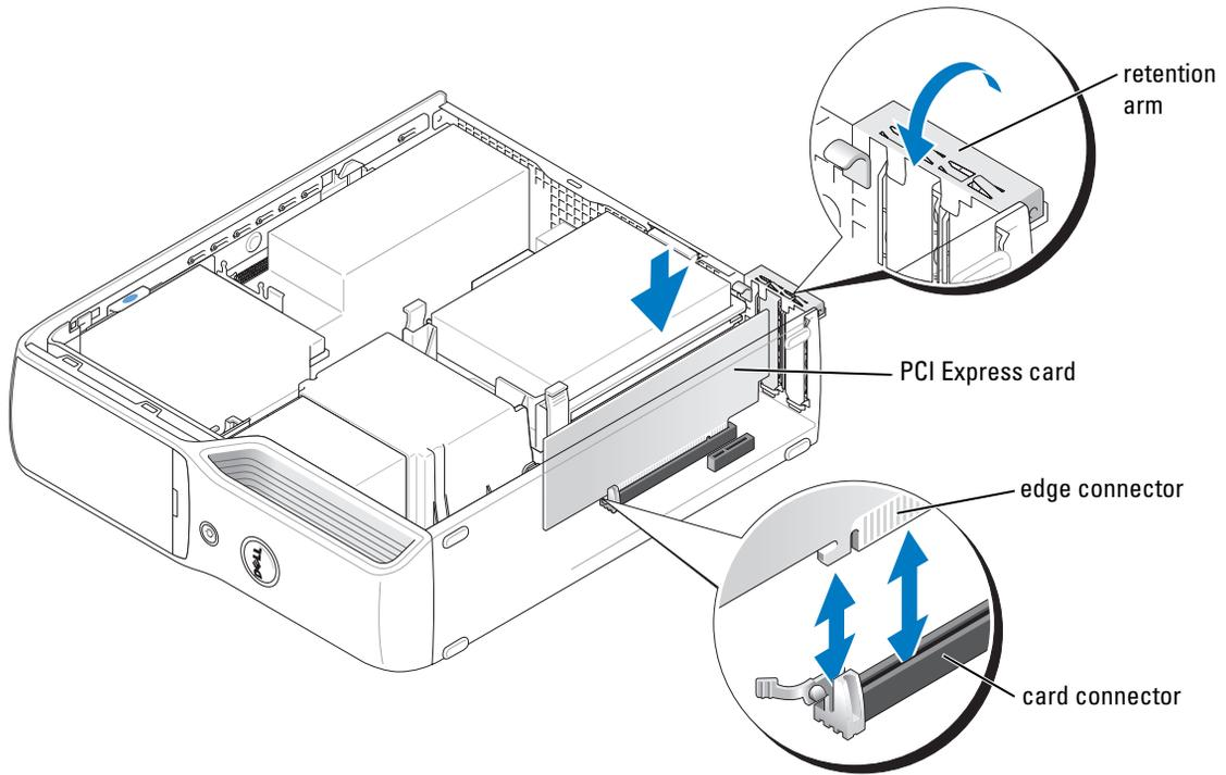
➡ **NOTICE:** Do not route card cables over or behind the cards. Cables routed over the cards can prevent the computer cover from closing properly or cause damage to the equipment.
