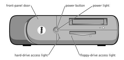
**HINT:** The front-panel door is removable; if you remove it or accidentally knock it off its hinges, it snaps back in place.
