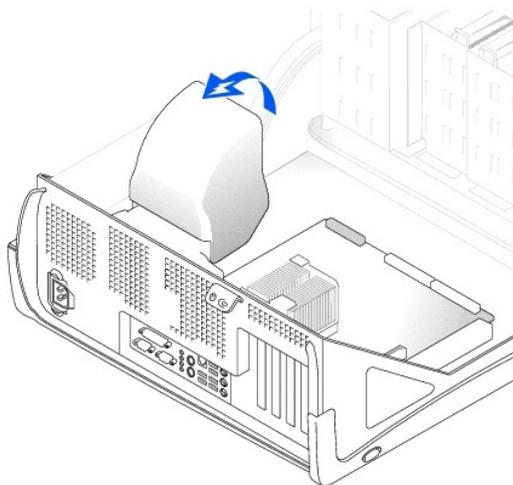
4. Remove the microprocessor heat sink:
