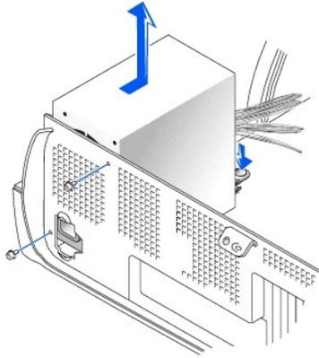
1. Disconnect the AC power cable from the back of the power supply.
