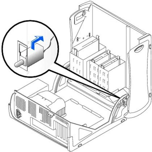
1. Disconnect the chassis intrusion switch cable connector from the control panel on the front of the chassis.
