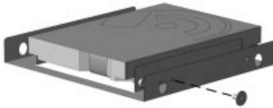
Inserting the High Hat Screw on the Right Side of the Bracket
