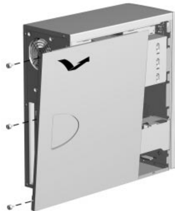
Removing the Minitower Computer Cover
