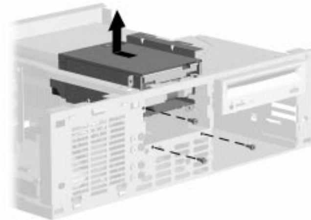
Removing the Drive Cage
