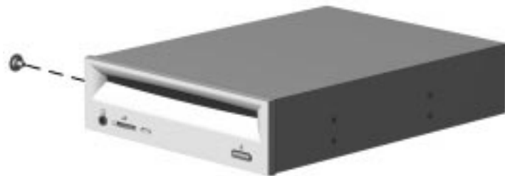
Installing the Wafer Screw into the CD-ROM Drive
